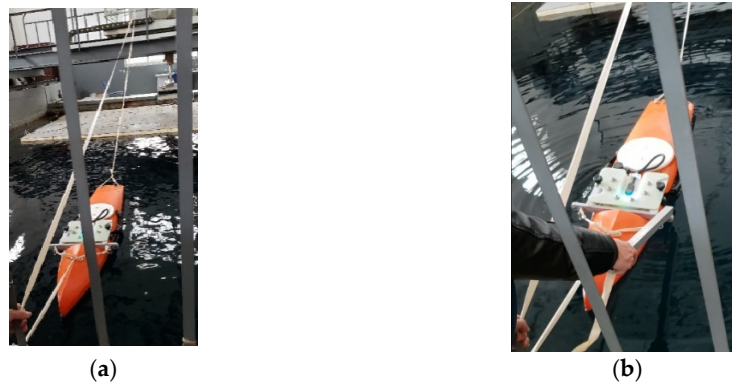
Figure 11. Pool test scenario diagram. (a) Method for moving the vessel. (b) Method for inducing vessel sway.
