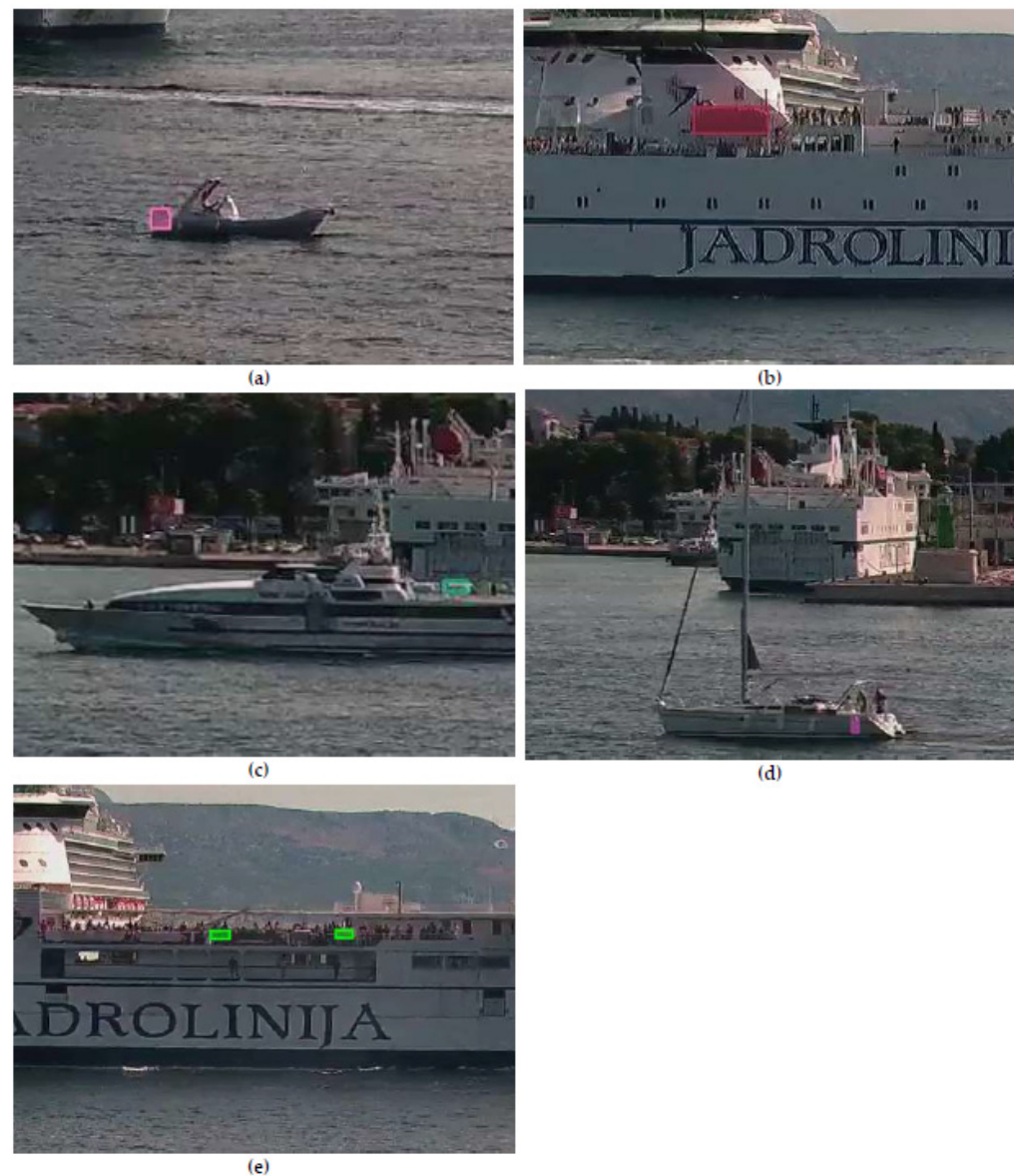
Figure 5. Example images of the vessels (enlarged for better viewing) with detected objects are as follows: (a) Speedboat 1 with ‘Motor cap’; (b) Large Ferry 1 with ‘Free-fall Lifeboat’; (c) Highspeed craft with ‘Large Life raft container’; (d) Sailboat with ‘Small fender’ vessels; (e) Ferry 2 with ‘Small Life raft container’.
