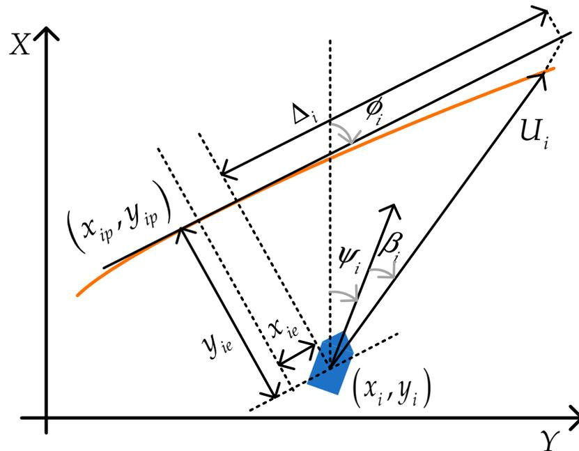
Figure 3. The geometry of LOS guidance.
