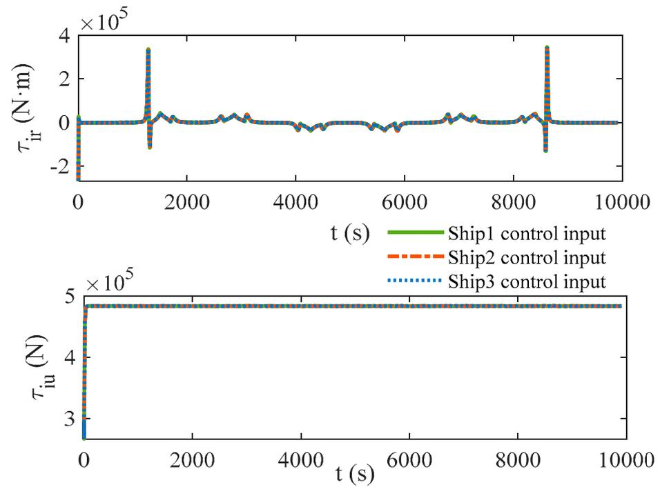
Figure 7. The control inputs of three ships.
