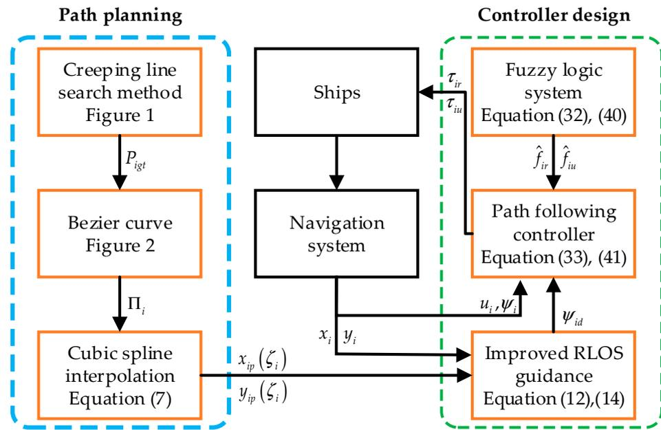
**Figure 4.** Diagram for cooperative maritime search control of multi-ship based on improved RLOS-guidance.
