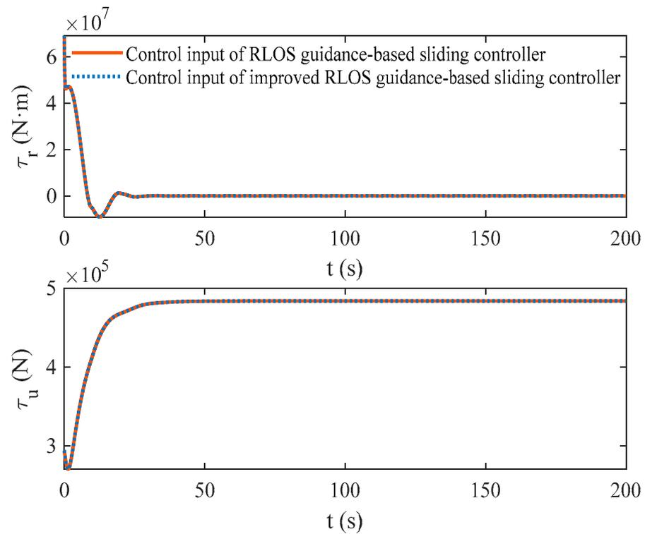
Figure 11. Control inputs of RLOS guidance-based sliding controller and improved RLOS guidance-based sliding controller.
