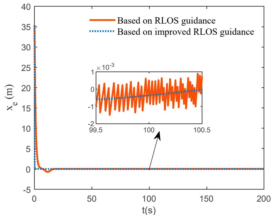
**Figure 12.** The comparison about  $x_e$  between RLOS guidance in [18] and improved RLOS guidance in this paper.
