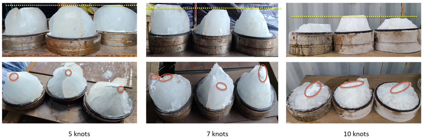
Figure 14. Fractures in the ice specimens after collision testing.
