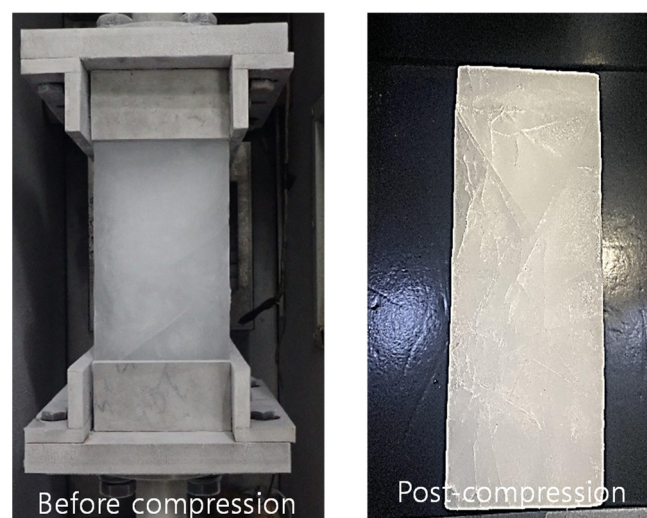
Figure 9. Fractured surface of an ice specimen after compression testing.
