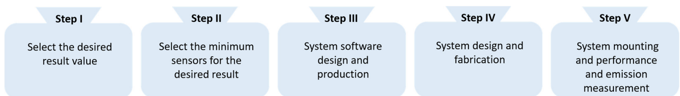
Figure 1. Methodology for designing a simplified performance-monitoring system.
