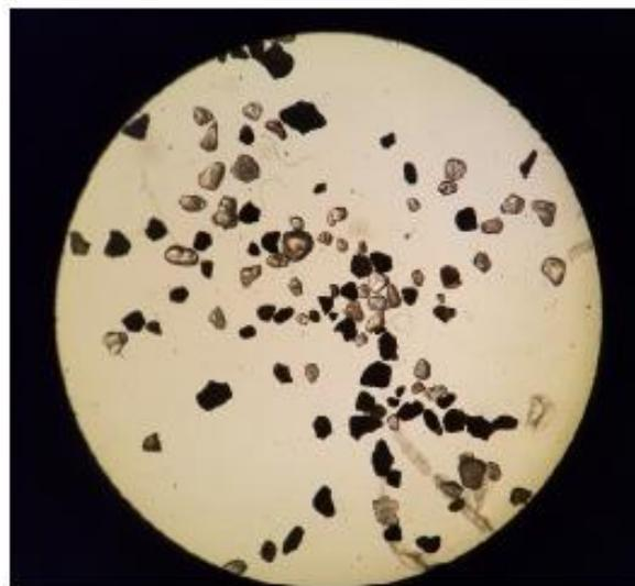
**Figure 5.** Sample of sand grains from Sand Point (ca. 55% stamp sands) under transmitted light from a microscope, showing the contrast between rounded natural sand (transparent quartz) and dark stamp sand grains (dark, irregular, slightly larger).
