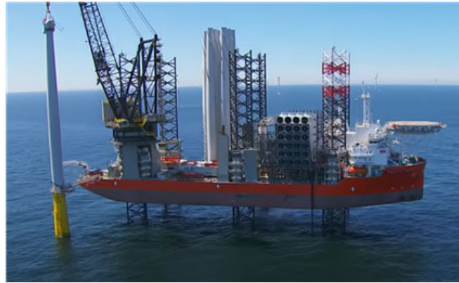
Figure 1. Operating WTIV of Swire Blue Ocean. ( https://splash247.com/cadeler-firms-up-scottish-offshore-wind-turbine-installation-deal/deal/ accessed on 15 May 2023).
