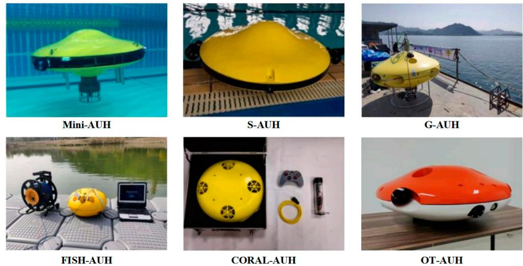
**Figure 8.** Development and Evolution of AUH Series Prototypes.
