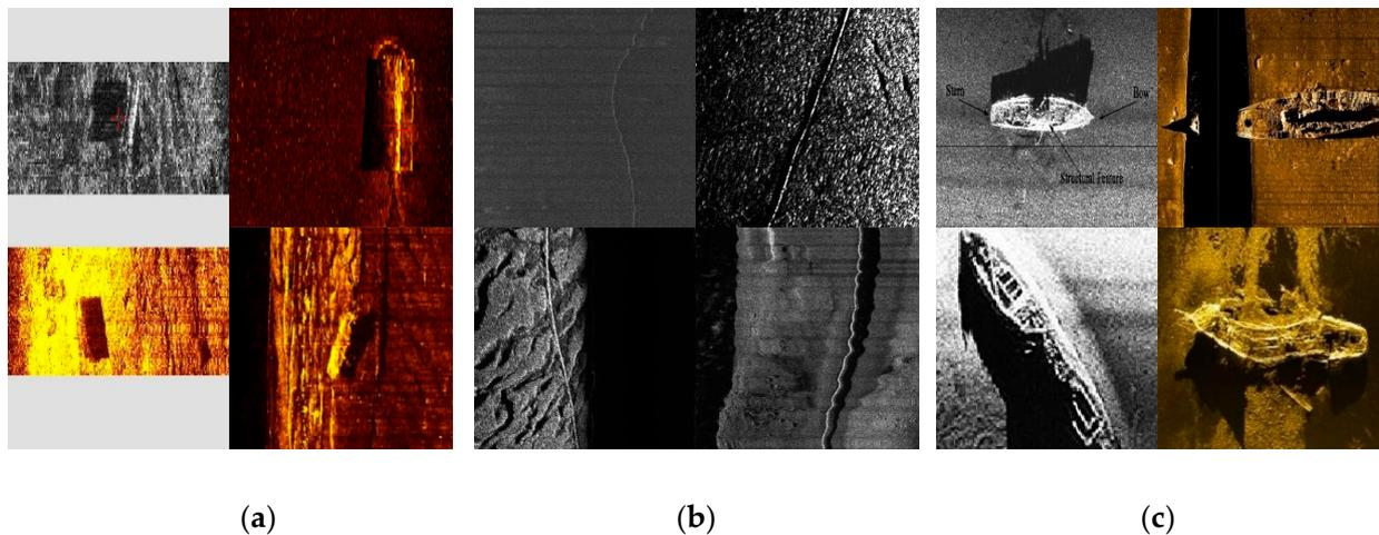
**Figure 5.** This is a sample training set for a part of the diffusion model. (a) Container; (b) pipelines; (c) shipwreck.
