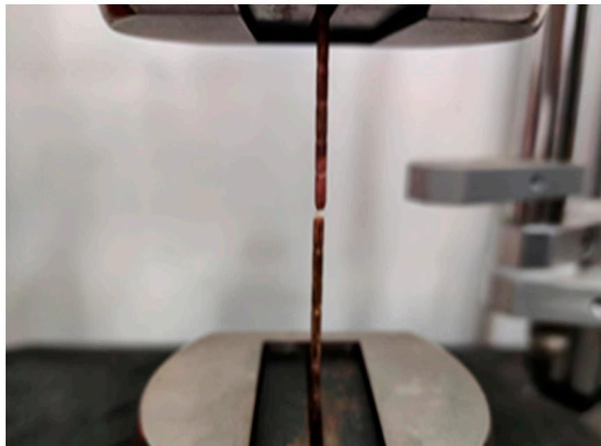
**Figure 20.** Broken area of mesh wire under the semi-immersed corrosion.
