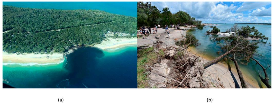
**Figure 1.** Inskip Point coastal flow slides: when coastal flow slides occur below the waterline, the coastline loses its support, and a portion of it slips seaward, creating a hole, the edges of which regress toward the coast. ((a): The Sunshine Coast Daily, 2015, (b): SBS news, 2015).
