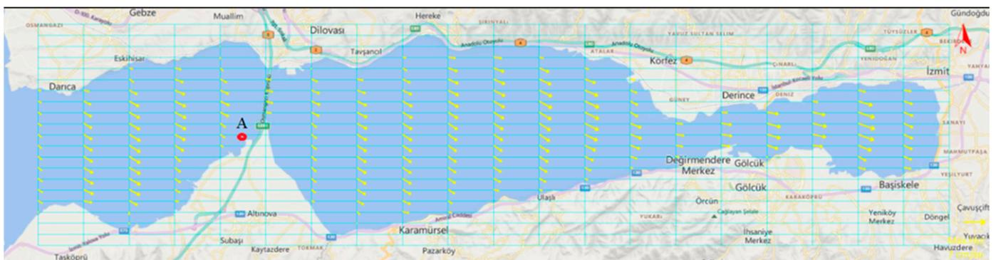
**Figure 15.** The pattern of the currents on the surface of the water at steady state with winds coming from the north-northwest at 10 m per second.
