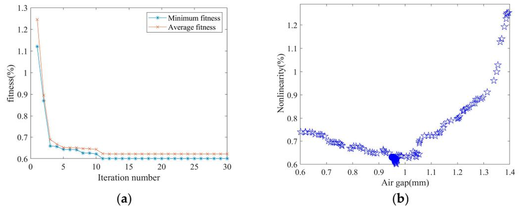
**Figure 10.** Sensor optimization simulations: (a) fitness value with iteration number; (b) linearity error vs. the air gap obtained in optimization design.
