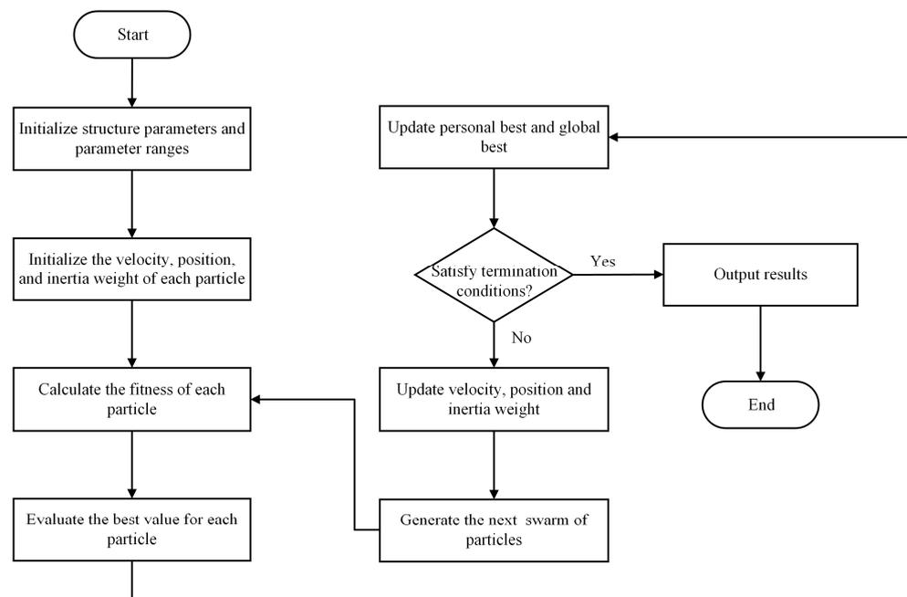
Figure 9. Flow chart of LINWPSO optimization process.
