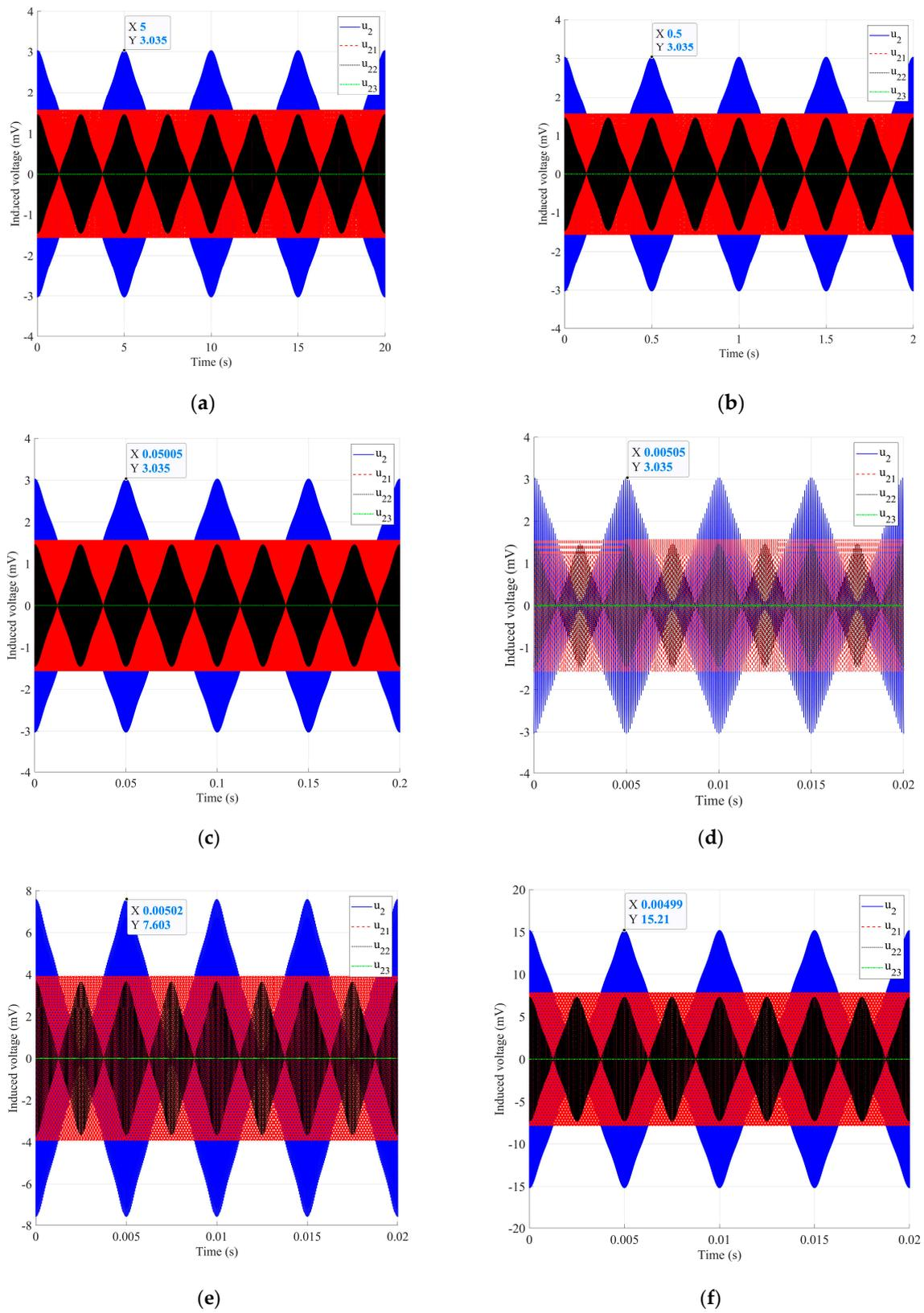
**Figure 8.** Simulation curves of induced voltage corresponding to different speeds and frequencies: (a)  $n_a = 1$  r/min,  $f_1 = 10$  kHz; (b)  $n_a = 10$  r/min,  $f_1 = 10$  kHz; (c)  $n_a = 100$  r/min,  $f_1 = 10$  kHz; (d)  $n_a = 1000$  r/min,  $f_1 = 10$  kHz; (e)  $n_a = 1000$  r/min,  $f_1 = 25$  kHz; and (f)  $n_a = 1000$  r/min,  $f_1 = 50$  kHz.
