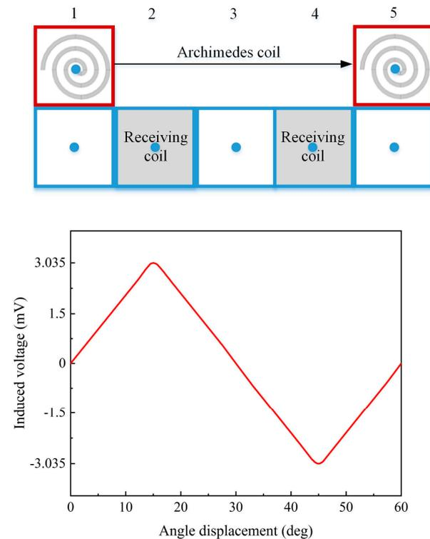
Figure 3. Induced voltage of receiving coils over one cycle.
