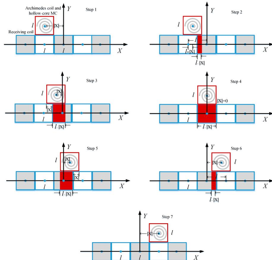
Figure 5. Relative motion diagram of coils.
