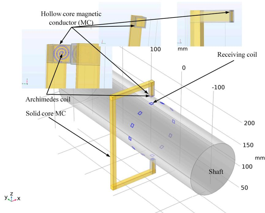
Figure 1. Sensor structure diagram.
