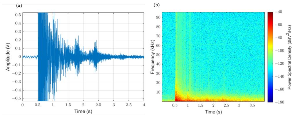
**Figure 3.** Details of an underwater explosion event recorded (a) in the temporary domain, with the Y-axis representing the output voltage of the electroacoustic chain and (b) in the time–frequency domain (obtained in  $\text{dBV}^2/\text{Hz}$ ). It is possible to observe how the acoustical signal exceeded the allowable full-scale input ( $\pm\sqrt{2} * 0.375 \text{ V}$ ) of the SAMARUC analog-to-digital converter.
