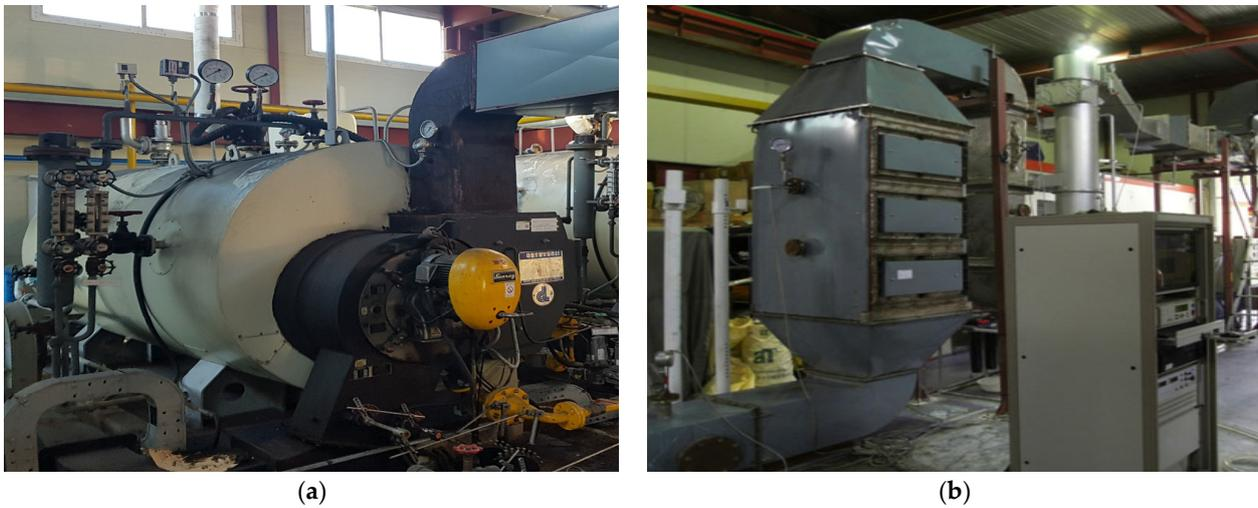
Figure 1. Photo of a 1.5-ton marine boiler using SCR systems: (a) 1.5-ton marine boiler; (b) SCR reactor.
