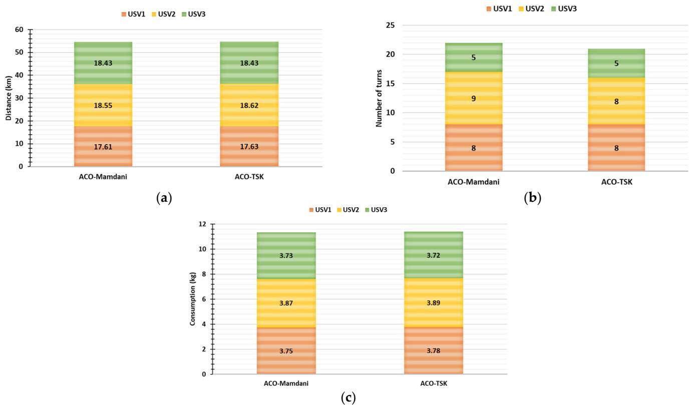
**Figure 8.** Cumulative results of ACO-Mamdani and ACO-TSK over the objective criteria: (a) distance; (b) number of urns; and (c) consumption for Case Study 1.
