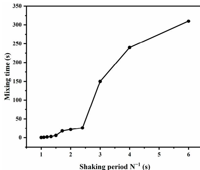
Figure 2. Relationship between mixing time and shaking period.
