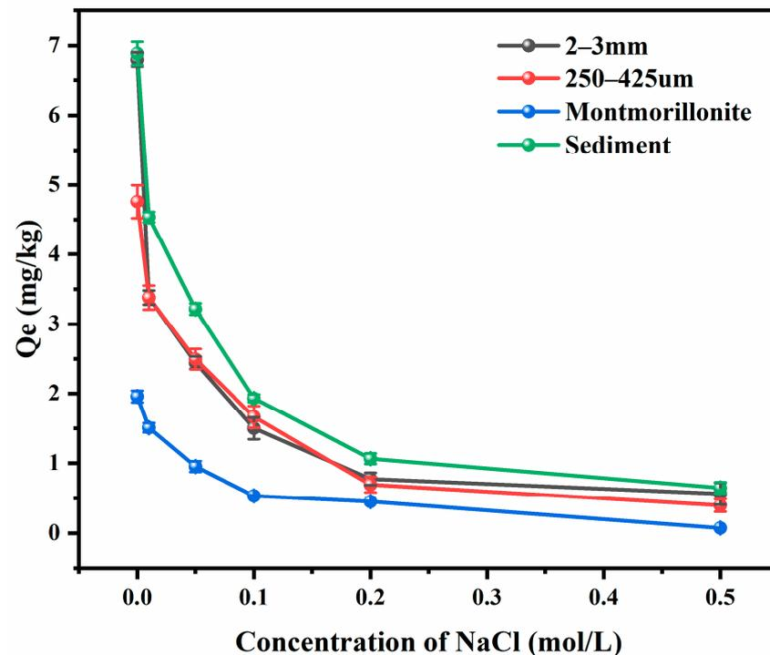
Figure 8. Adsorption of SDZ on different sediments under different salinity at  $Re = 7500$ .
