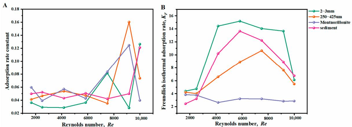
**Figure 6.** Relationship between Reynolds number and adsorption coefficients, (A) adsorption kinetic constant and (B) Freundlich coefficient.
