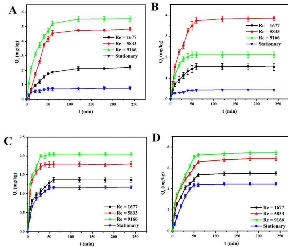
**Figure 4.** Variation of adsorption amount with time under different regimes on (A) 2–3 mm quartz sand (B) 250–425  $\mu\text{m}$  quartz sand (C) montmorillonite and (D) sediment sample.
