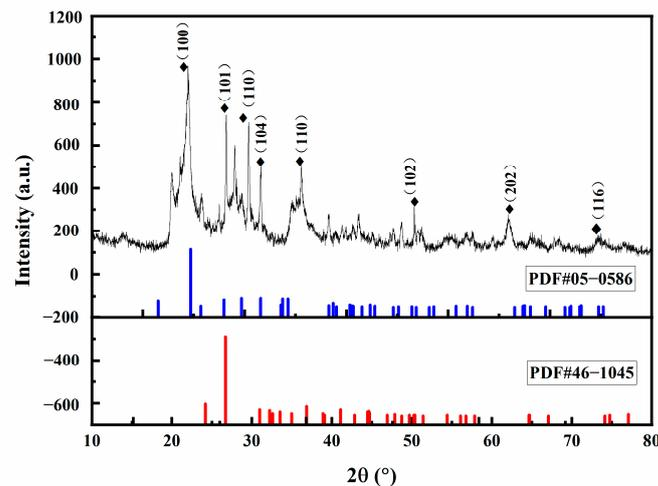
**Figure 1.** XRD characterization of sediments.
