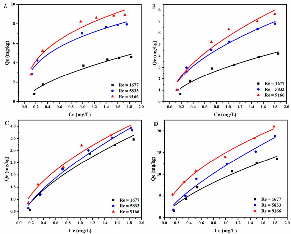
**Figure 5.** Relationship between equilibrium concentration and adsorption capacity with Freundlich model fitting under different hydrodynamic conditions on (A) 2–3 mm quartz sand, (B) 250–425  $\mu\text{m}$  quartz sand, and (C) montmorillonite. (D) Sediment sample.
