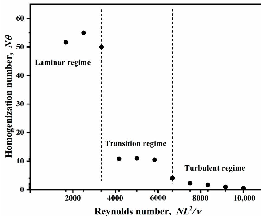
Figure 3. Relationship between Reynolds number and homogenization number.
