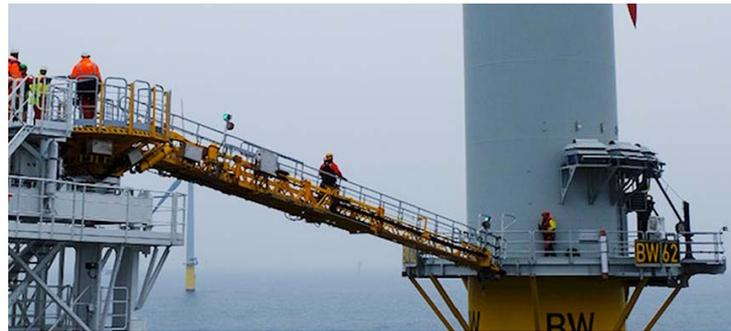
**Figure 1.** The three-DOF serial gangway.
