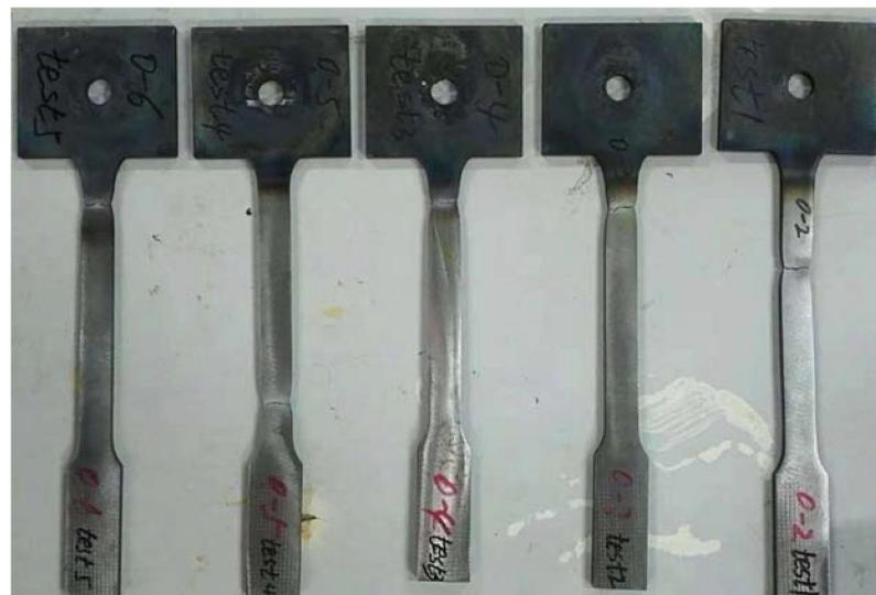
**Figure 3.** Failure of the quasi-static test specimen.
