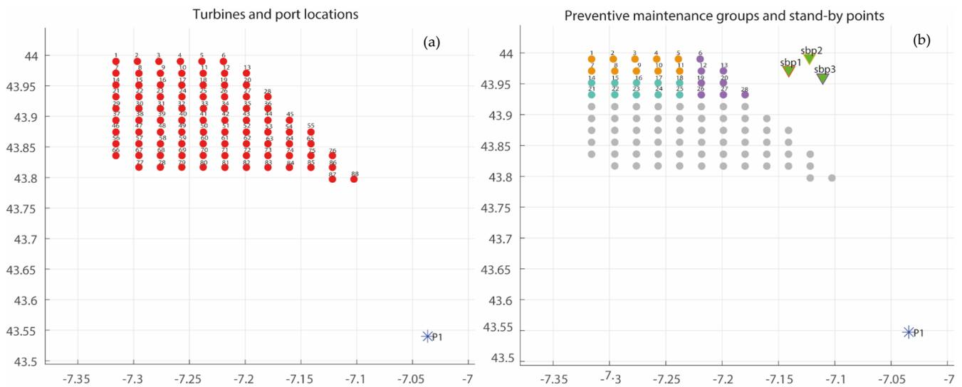
**Figure 2.** (a) Ribadeo floating wind farm layout (b) maintenance planning and possible offshore base locations. The asterisk symbol represents the port location.
