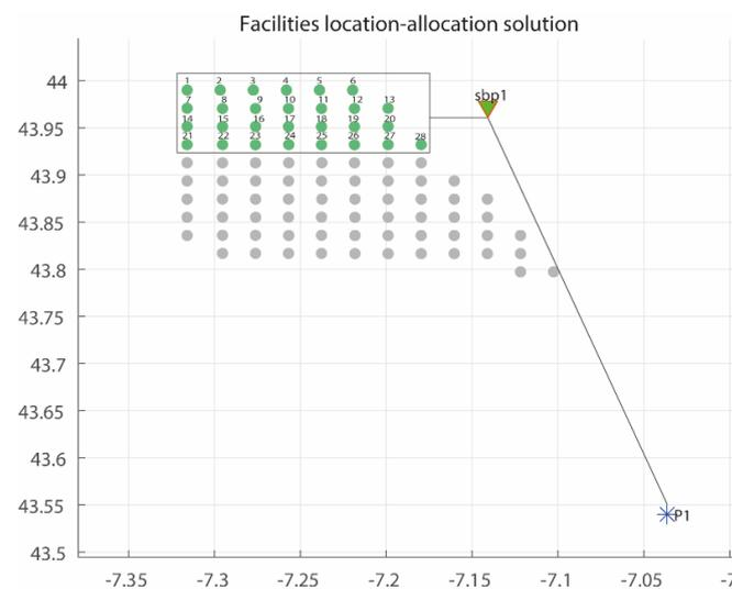
**Figure 3.** Facility location–allocation solution, where the green dots mean that all the turbines are allocated to the chosen stand-by point.
