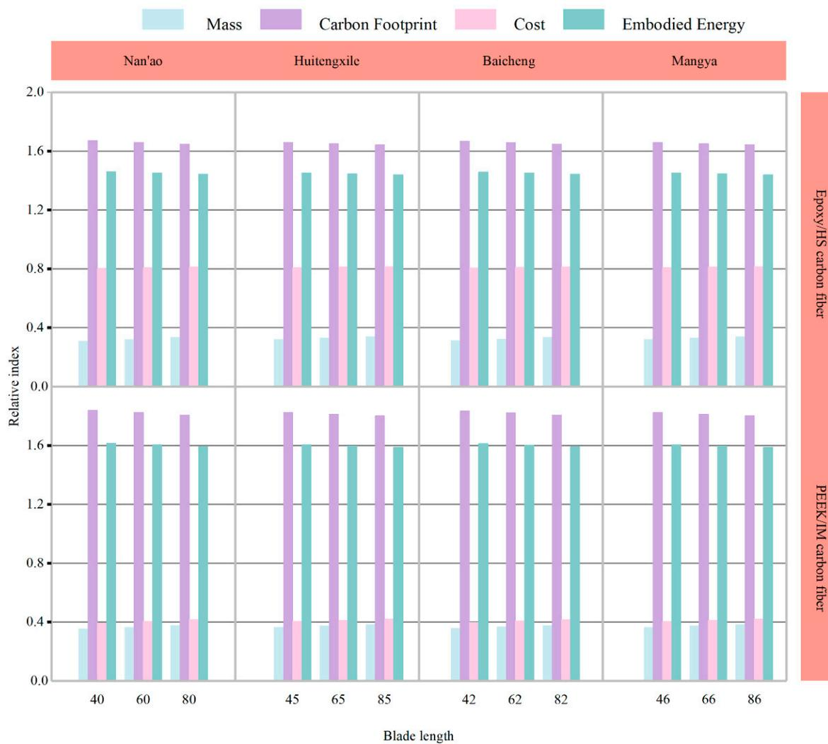
**Figure 6.** Economic comparison between carbon fiber blade and traditional glass fiber blade. Note: Only the cost of purchasing materials is considered, and the difficult processing, transportation, storage, import tax rate, and other costs of carbon fiber composites are not considered. Only the material mass of the central part of the wind turbine blade is considered.
