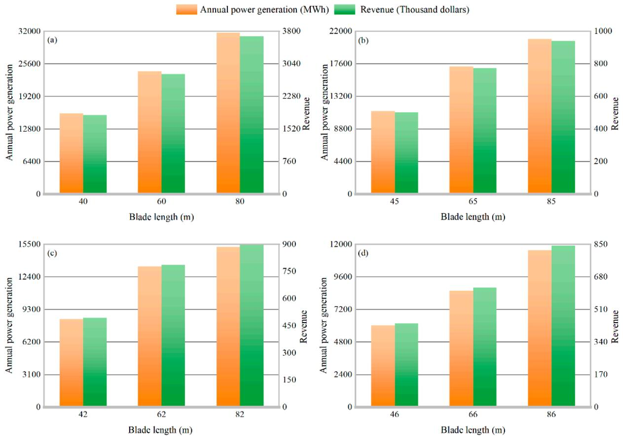
**Figure 5.** Comparison of energy efficiency after increasing the blade length in different regions: (a) Guangdong Nan’ao; (b) Nei Monggol Huitengxile; (c) Jilin Baicheng; (d) Qinghai–Tibet Plateau Mangya. Notes: The feed-in tariffs for Nan’ao, Huiteng Xile, Baicheng, and Qinghai–Tibet Plateau are CNY 0.75 (USD 0.116), CNY 0.29 (USD 0.045), CNY 0.38 (USD 0.059), and CNY 0.47 (USD 0.073), respectively.
