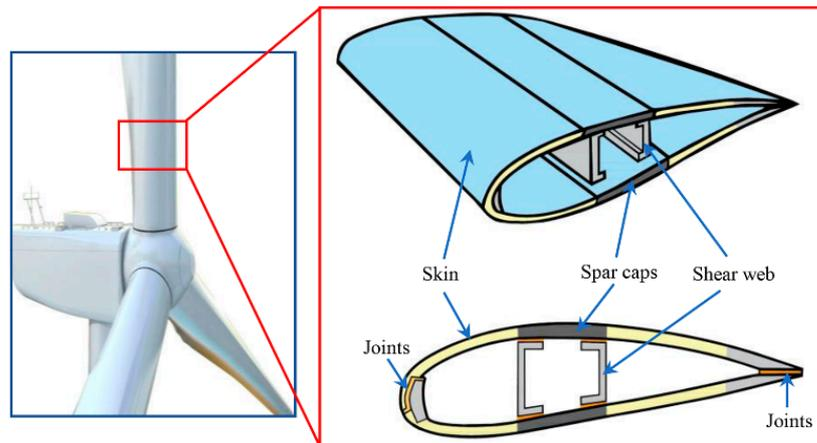
Figure 1. Structural drawing of wind turbine blade.
