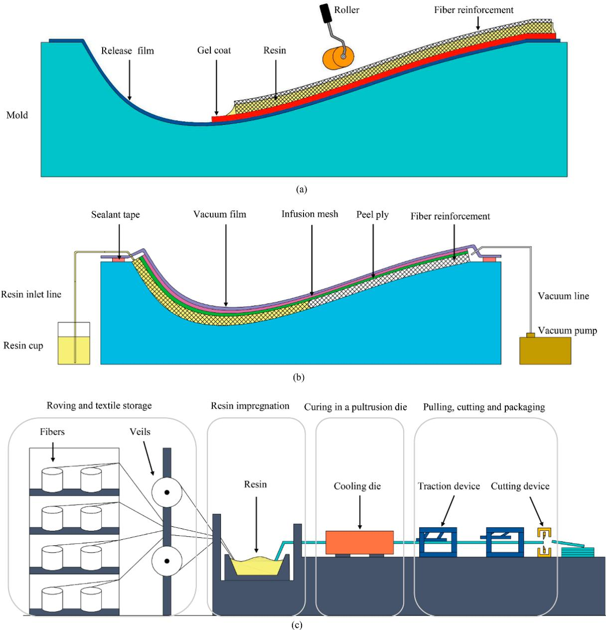
**Figure 9.** The main stages of manufacturing technology for wind turbine blades. (a) Stage 1: hand lay-up; (b) Stage 2: vacuum infusion process; (c) Stage 3: pultrusion process.
