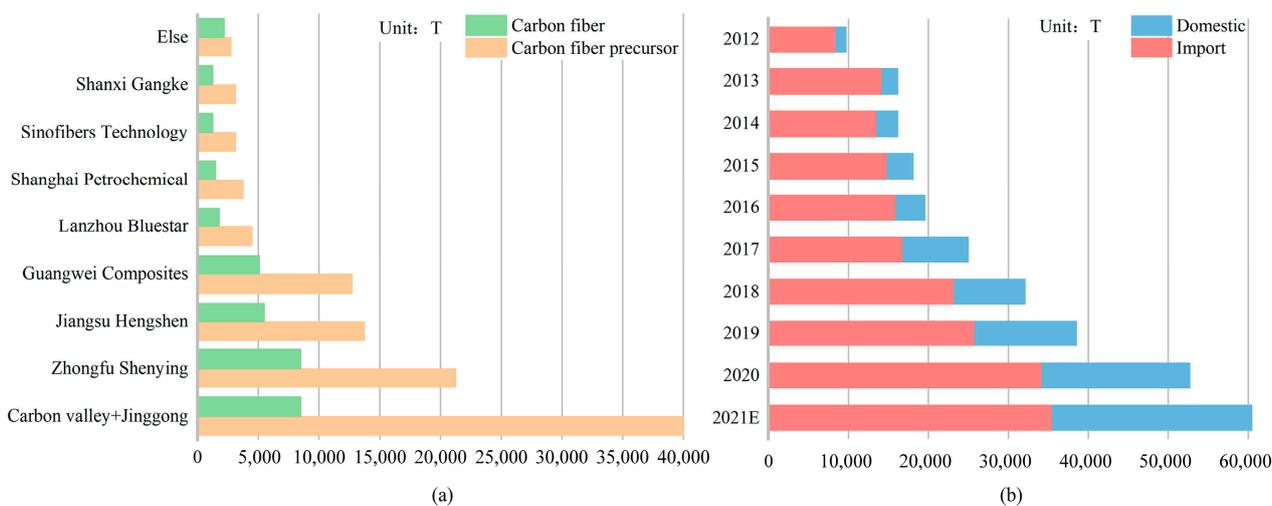
**Figure 7.** Carbon fiber production and demand in China. (a) China’s CF precursor and CF operating capacities in 2020 by manufacturer; (b) Chinese demand for carbon fibers.
