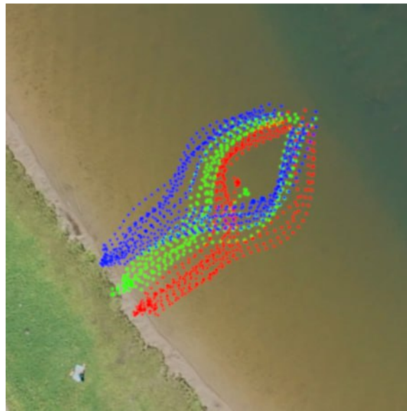
Figure 19. Trajectories of the mini-boats in group motion considering obstacle avoidance. Blue, red and green dots corresponding to the trajectory of the first, second and third robot in the group accordingly.
