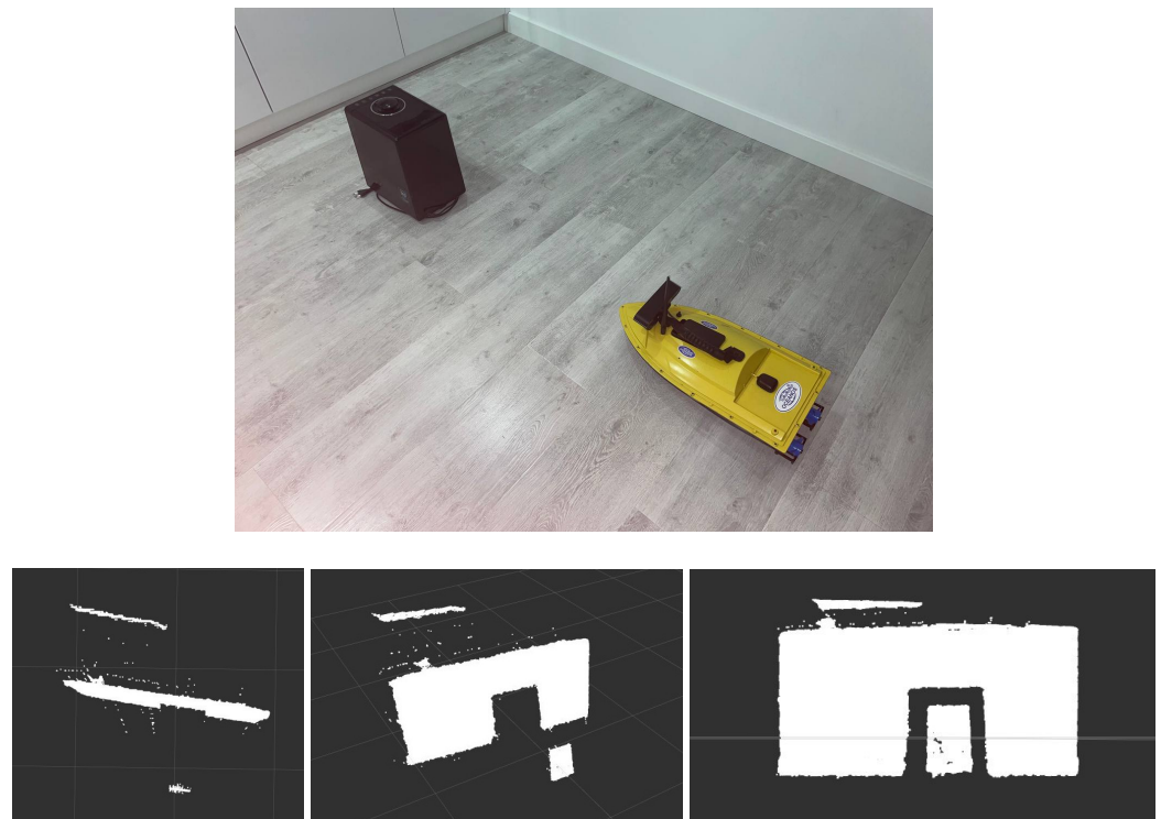
Figure 16. Astra Pro Realsense RGBD Depth Camera point cloud viewing experiment with SMTU.
