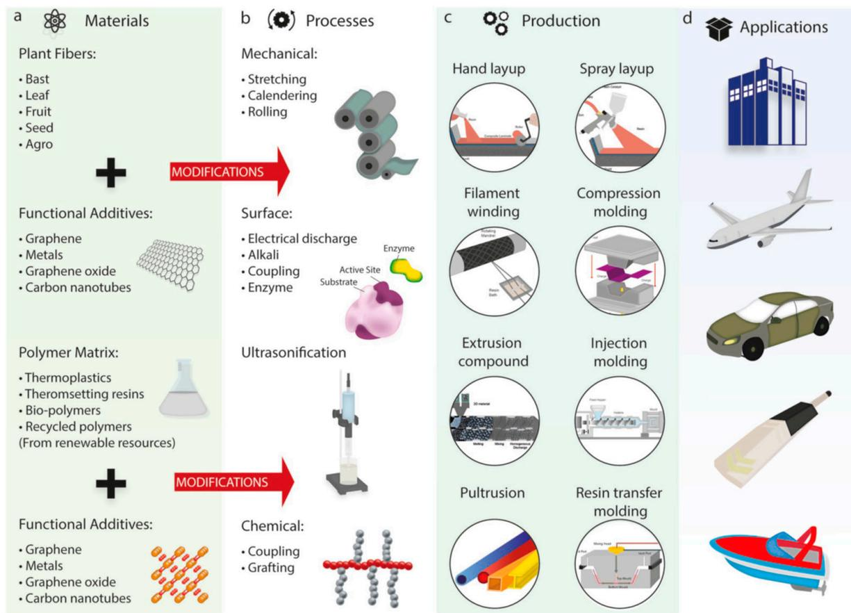
**Figure 8.** Sustainable FRP composites: (a) materials, (b) modification processes, (c) composite manufacturing methods, and (d) applications of fibre-reinforced composites [55].
