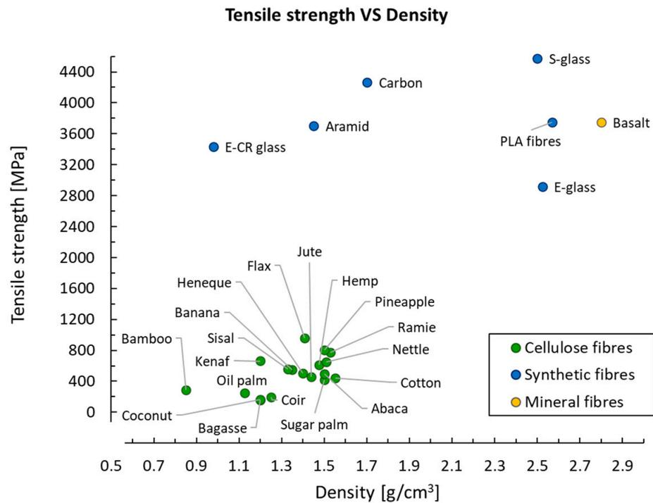
Figure 6. Map of the tensile strength against density for several cellulose, synthetic, and mineral fibres. Data from [52,55,58–63].
