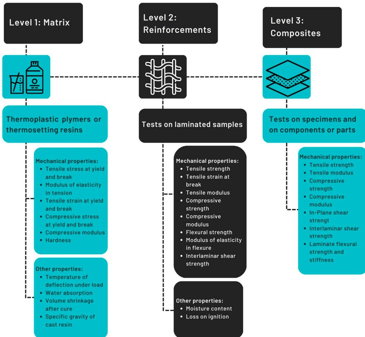
Figure 12. Summary of the properties to be assessed for composites to be used in marine structures, according to classification societies.
