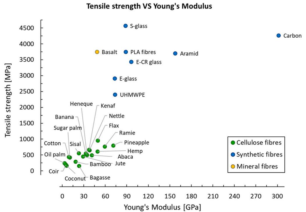
Figure 5. Map of the tensile strength against Young’s modulus for several cellulose, synthetic, and mineral fibres. Data from [52,55,58–63].
