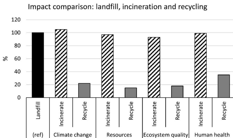
Figure 1. The impact comparison of landfill disposal, incineration, and recycling [24].
