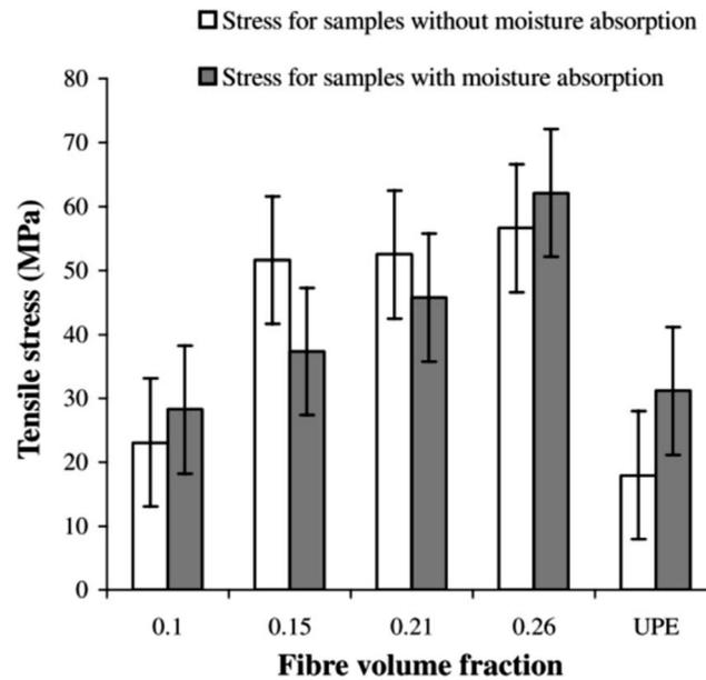
Figure 9. Moisture effect on the tensile strength of hemp/UP composites (reproduced from [56]).
