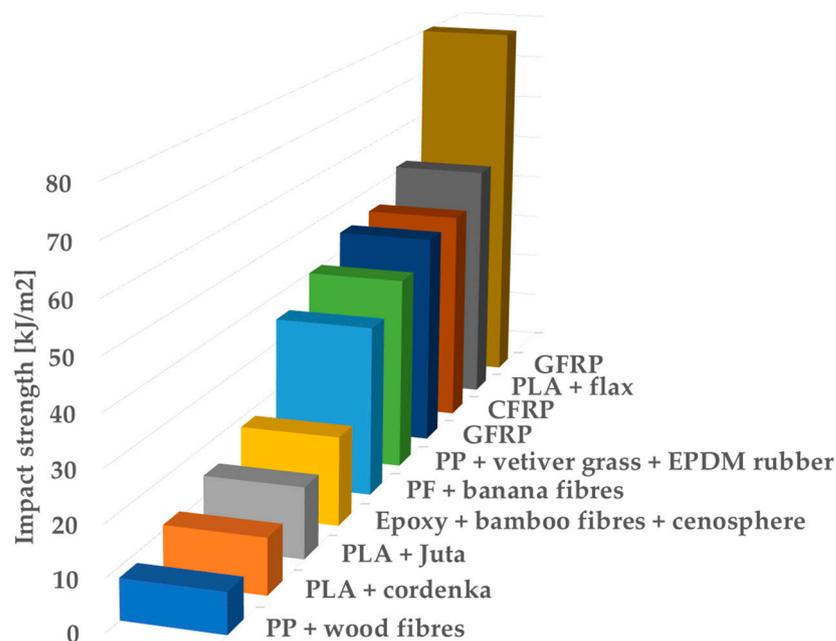
Figure 10. Impact strength of bio-based and traditional composites. Data from Refs. [84–91].
