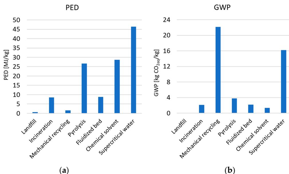
**Figure 2.** Averaged (a) PED and (b) GWP of the main EoL methods for composites, according to data from [16,26–33].
