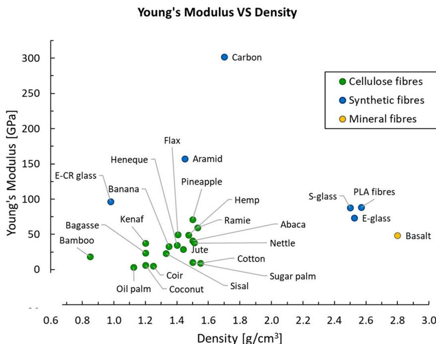
**Figure 7.** Map of the Young’s modulus against density for several cellulose, synthetic, and mineral fibres. Data from [52,55,58–63].
