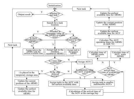
Figure 6. Flow chart of ARMG and AGV task allocation.
