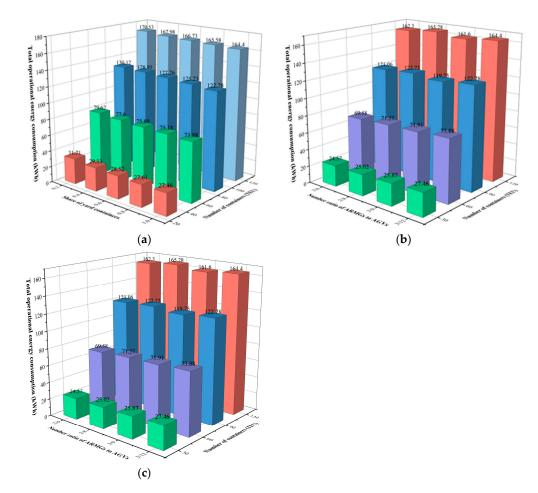
Figure 13. (a) Variation in energy consumption for different containers and ratio of "transshipment" containers with 3 ARMGs and 12 AGVs; (b) Variation in energy consumption for different containers, ARMG, and AGV configurations with all "transshipment" containers; (c) Incremental energy consumption for yard containers ratios and different ARMG to AGV ratios for 120 TEU.
