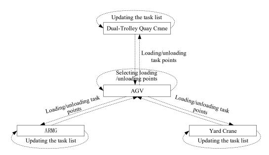
Figure 2. Constraint relationship between ARGC, AGV, AQC, and YC in the rail-in-port model.
