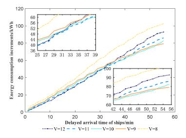
Figure 12. Variation in energy consumption for different ship delay times and number of AGVs.
