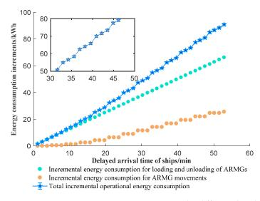
Figure 11. Variation in energy consumption under different ship delay time.
