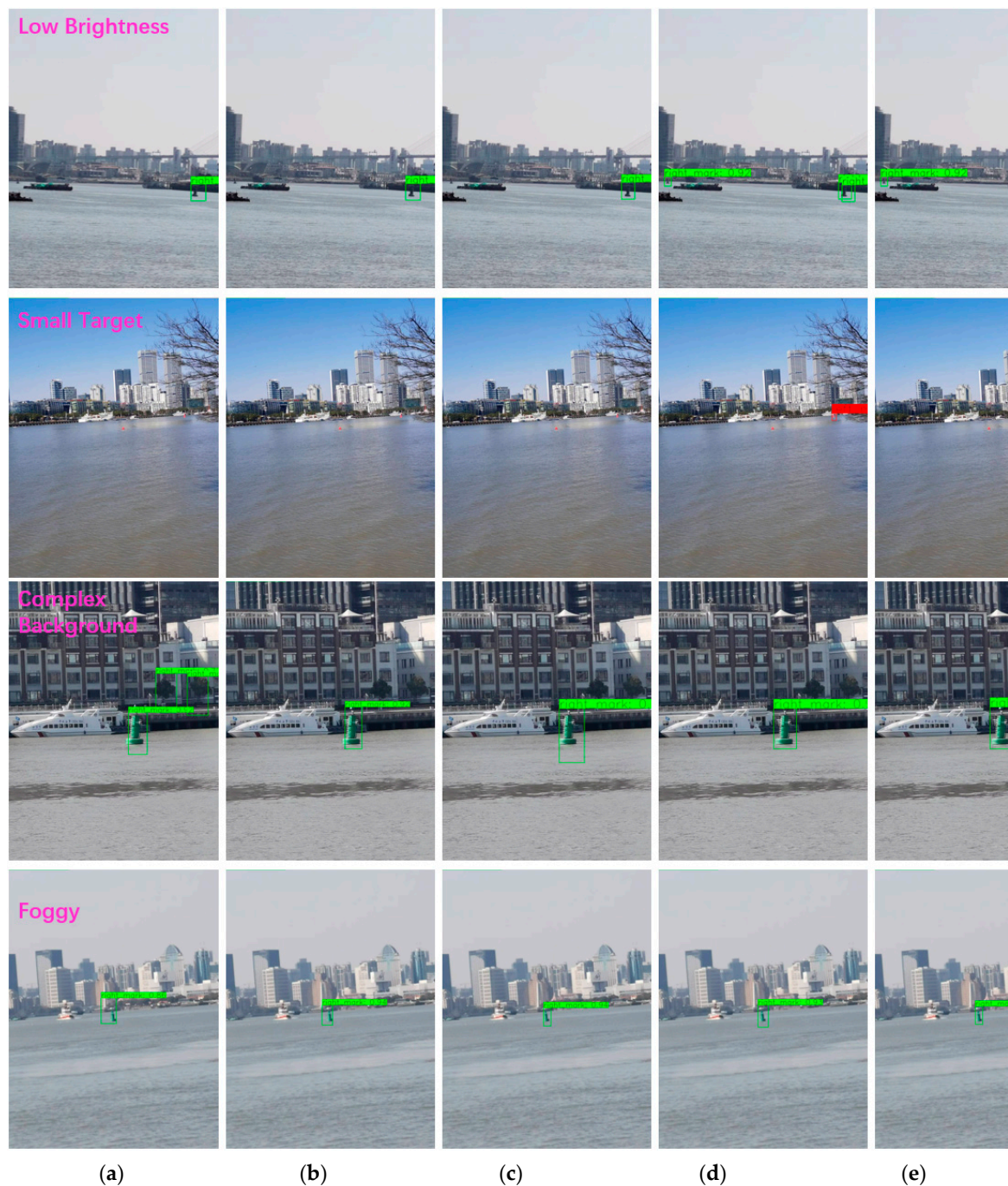
Figure 9. (a) YOLOv4-tiny; (b) YOLOv4; (c) Mask-RCNN; (d) Faster-RCNN; (e) NM-YOLOv4(ours). In four different scenarios (complex background, foggy, low brightness, and small target), test results of algorithms YOLOv4-tiny, YOLOv4, Faster-RCNN Mask-RCNN, and NM-YOLOv4(ours).
