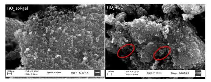
Figure 3. SEM images of (a) TiO<sub>2</sub> sol-gel, and (b) TiO<sub>2</sub>-rGO, with the rGO sheets highlighted in red.
