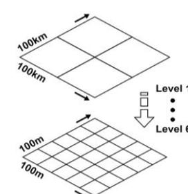
The maritime traffic distribution characteristics at a specific site may be quantitatively identified when the analysis range in Korean coastal waters is gridded using the grid-type marine information management system of the KHOA. Moreover, the system can be efficiently applied to related studies, such as securing compatibility with chart-size variations, by employing data based on grid-type data.
