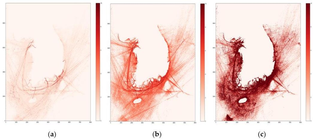
**Figure 10.** Results of visualization of marine traffic distribution by AIS data: (a) maritime traffic status based on LOA characteristics; (b) maritime traffic status based on SOG characteristics; (c) maritime traffic status based on frequency characteristics.
