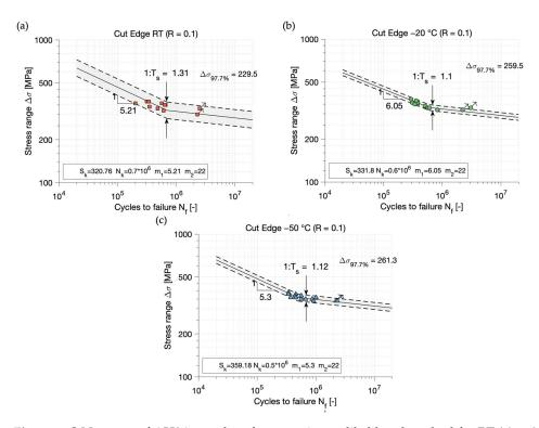
**Figure 6.** S-N curves of AH36 cut edges from maximum likelihood method for RT (**a**), -20 °C (**b**) and -50 °C (**c**).
