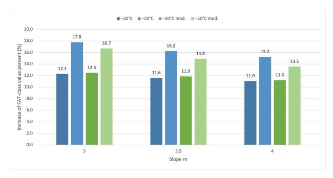
**Figure 10.** Increase in the FAT-class value in percent of tested AH36 cut edges at sub-zero temperatures compared to RT and of modified test series compared to RT modified. In the modified test series, the nominal stresses in the cross sections at the actual crack locations are used instead of the nominal stresses at the smallest cross sections.
