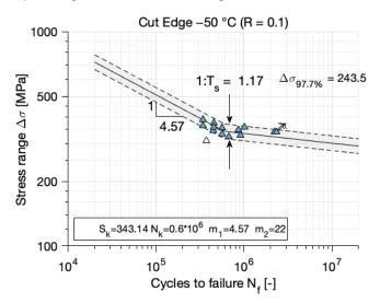
**Figure 9.** S-N curve of AH36 cut edges for test results at -50 °C with modified stress ranges evaluated with the maximum likelihood method. The white triangle shows the outliner.
