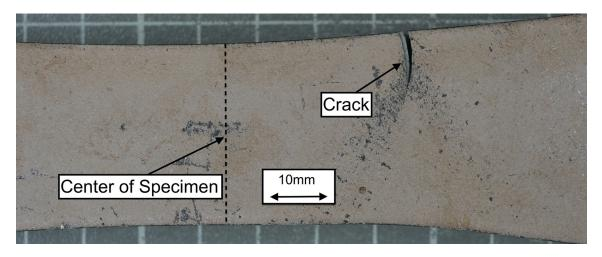
Figure 8. Specimen where the crack position is not at the smallest cross section.
