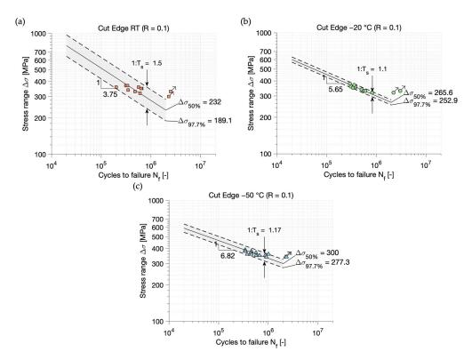
**Figure 5.** S-N curves of AH36 cut edges from linear regression for RT (a), -20 °C (b) and -50 °C (c).
