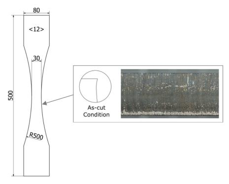
Figure 2. Specimen dimension and cut condition, modified from [12].
