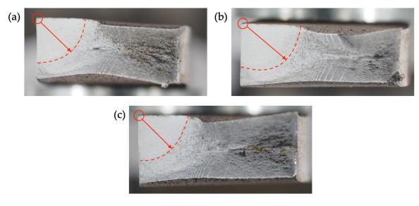
**Figure 7.** Fracture surface of AH36 cut edges tested at temperatures of RT (**a**),  $-20 \degree \text{C}$  (**b**) and  $-50 \degree \text{C}$  (**c**), with location of crack initiation and direction of crack propagation.
