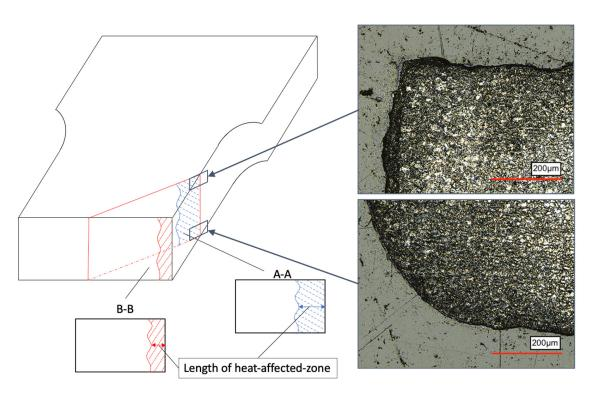
**Figure 3.** Microstructure of polished inclined cross section. Top side edge with sharp corner (flame entry) and more round edge on bottom side.
