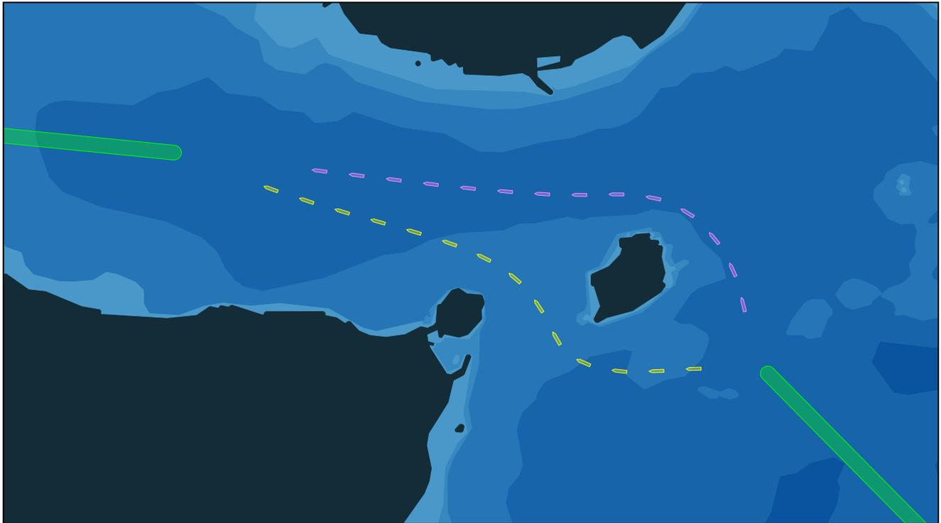
**Figure 13.** Path following simulation example, based on a simple line-of-sight guidance controller.
