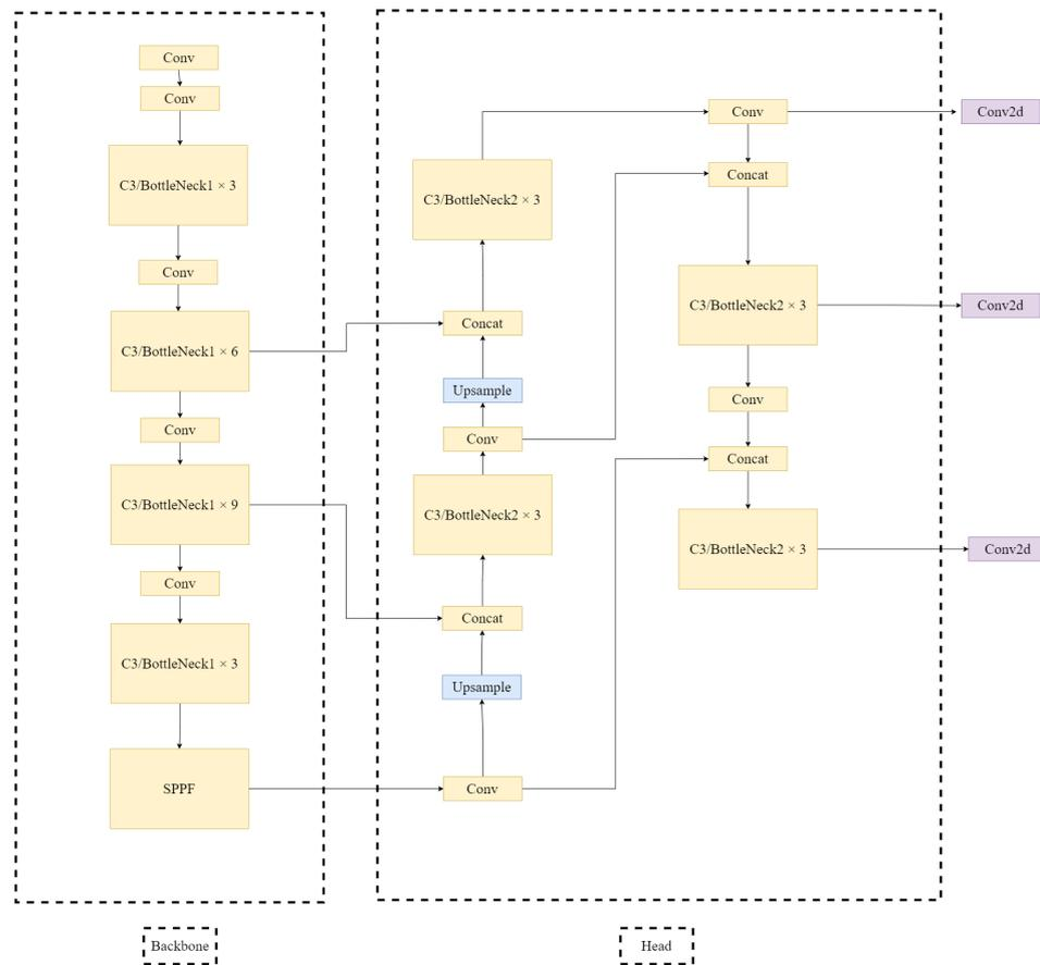
Figure 5. YOLOv5 structure.
