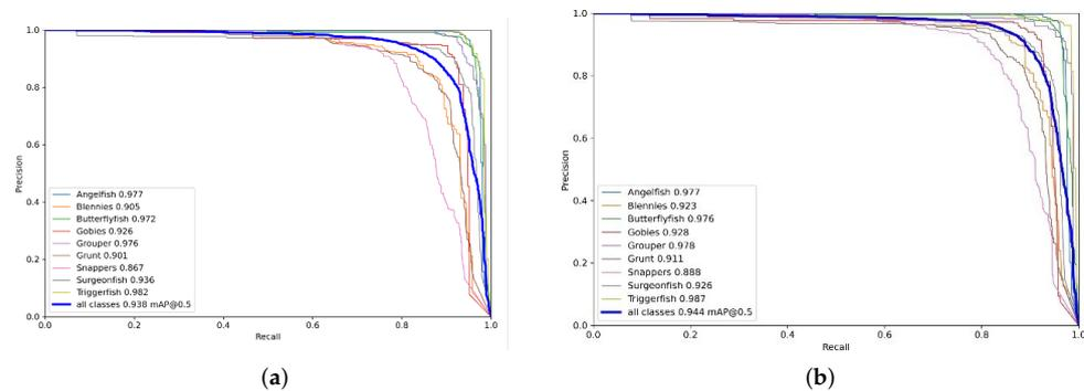
Figure 18. PR curve of the improved model. (a) PR curves for model S-Head-Ghost-Fish9. (b) PR curves for model S-SE-HorBlock-Head-Ghost-Fish9.
