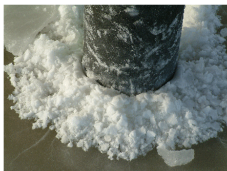
Figure 4. Crushing failure of sea ice on the vertical pile structure in field data of the Bohai Sea.
