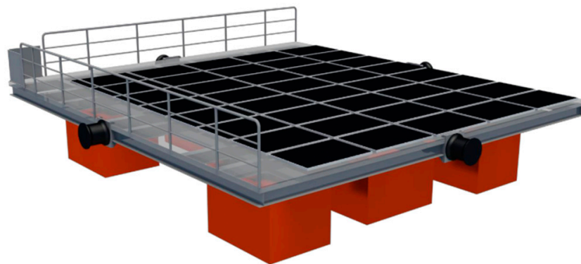
Figure 9. Square floating platform developed by the Norwegian company New Energy [96].
