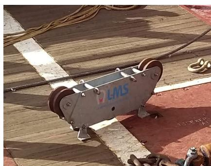
**Figure 2.** Running Line Monitor (RLM) to measure towline tension.
