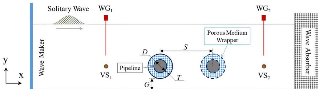
Figure 5. Layout for solitary wave impinging on the submarine pipeline encased in porous media.
