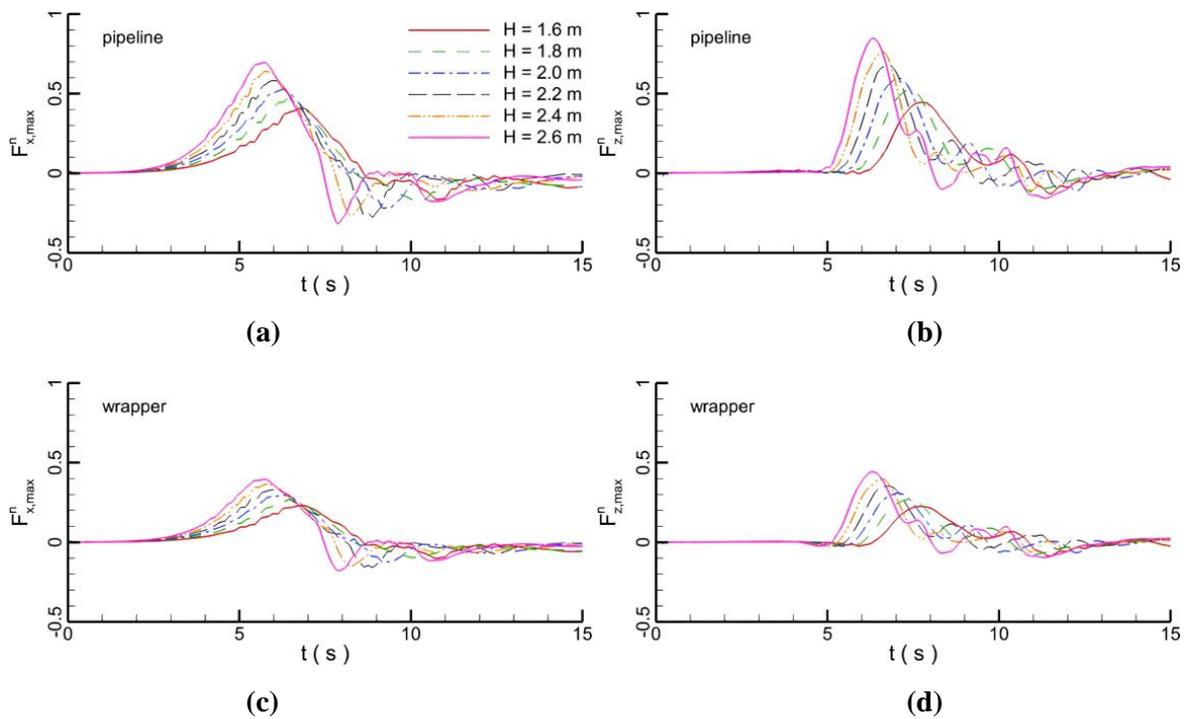
**Figure 24.** The temporal evolutions of forces on the pipeline and wrapper; (a) Horizontal maximum force on pipeline; (b) Vertical maximum force on pipeline; (c) Horizontal maximum force on wrapper; (d) Vertical maximum force on wrapper.
