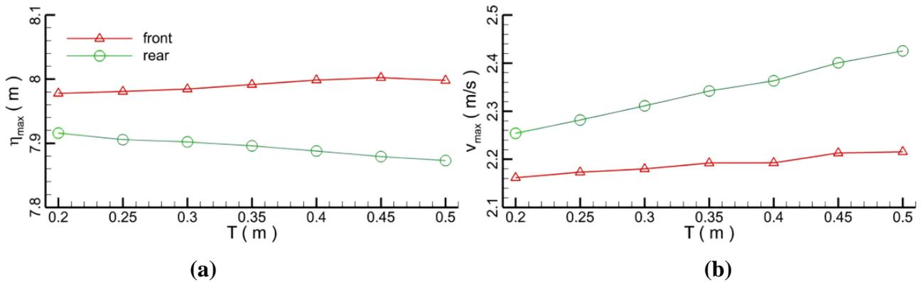
**Figure 14.** Comparisons of the maximum elevations and velocities in front and rear of the pipelines with different wrapper thicknesses; (a) free surface elevation (note: original water depth is 6 m); (b) velocity.
