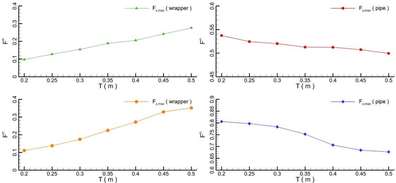
**Figure 15.** Hydrodynamic forces on the pipeline and wrapper.
