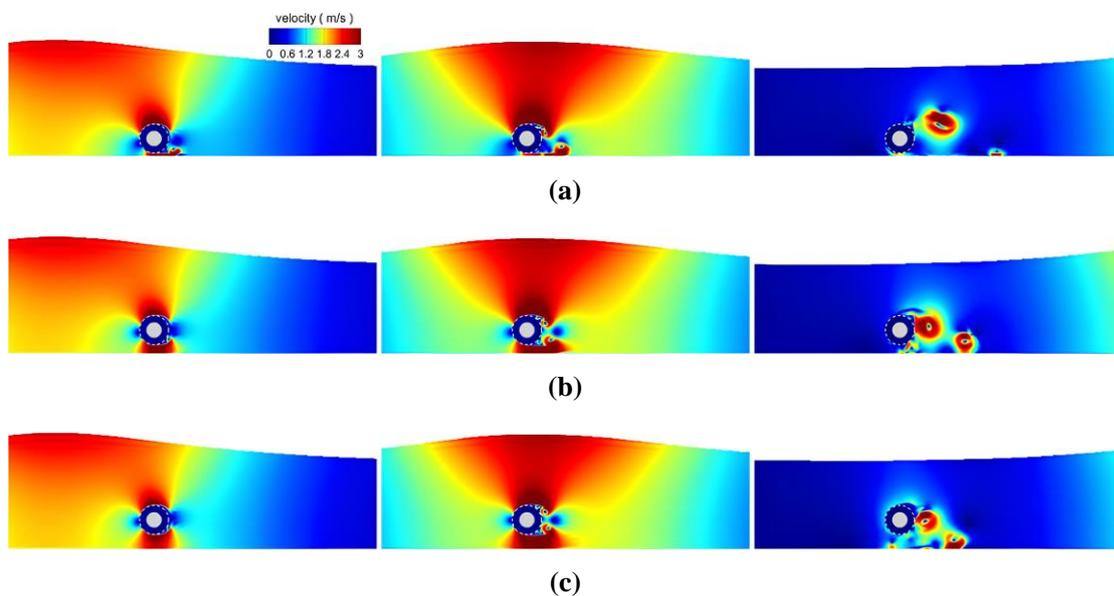
**Figure 16.** The velocity contours of the flow fields under different gaps; (a)  $G = 0.2$  m; (b)  $G = 0.6$  m; (c)  $G = 1.0$  m. Left to right: 6.3 s, 7.2 s, and 10.2 s. Left to right: arrival, stay, departure.
