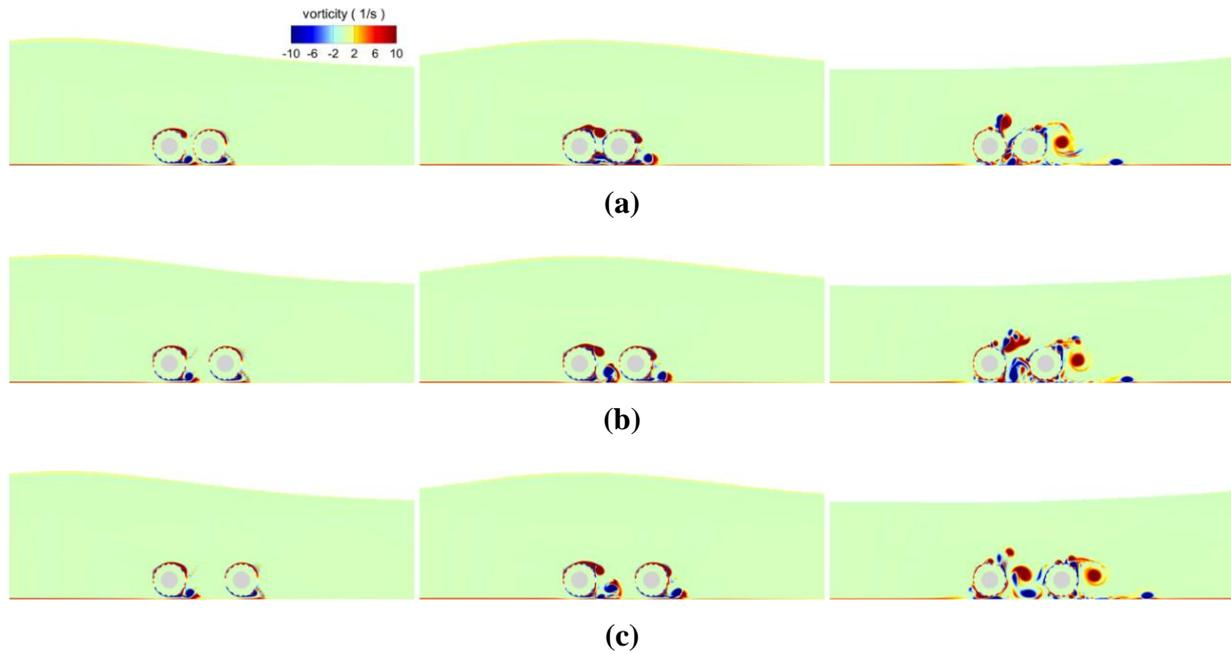
**Figure 20.** The vorticity contours of the flow fields under different porosities; (a)  $S = 2.5$  m; (b)  $S = 3.5$  m; (c)  $S = 4.5$  m. Left to right: 6.3 s, 7.2 s and 10.2 s.
