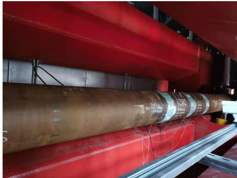
Figure 16. Full-size SCR test specimen.
