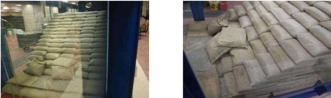
**Figure 19.** Configuration with slope 1:1.5. Uplift and movement of some elements in the stability test with  $H = 0.20$  m,  $T = 1.5$  s and  $h = 0.40$  m.
