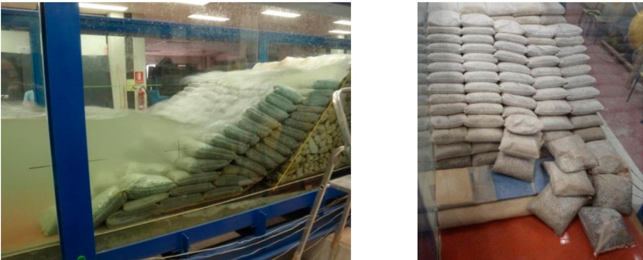
**Figure 18.** Configuration with slope 1:1. Instability of the structure in the stability test with  $H = 0.20$  m,  $T = 2.0$  s and  $h = 0.61$  m.
