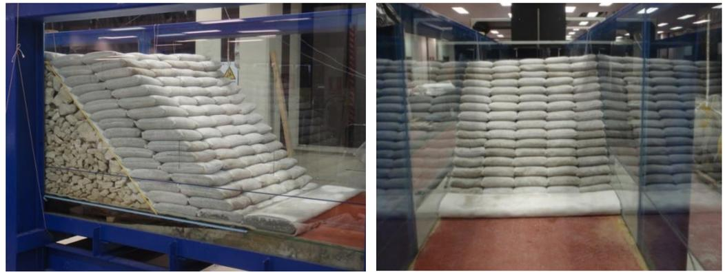
**Figure 5.** GSC revetment structure with a slope of 1:1 (lateral and front views).
