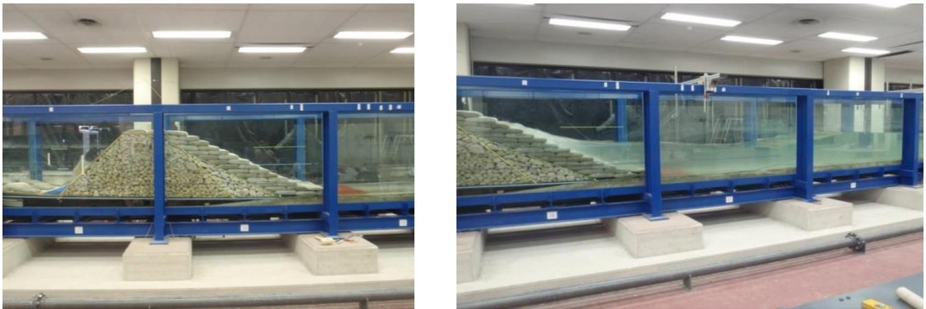
**Figure 6.** GSC revetment structure with a slope of 1:2.
