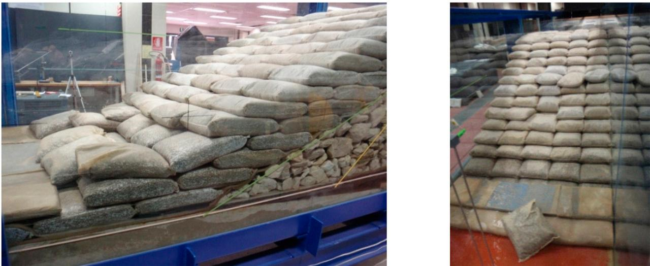
**Figure 20.** Configuration with slope 1:2. Sliding of some elements in the stability test with  $H = 0.20$  m,  $T = 2.0$  s and  $h = 0.40$  m (left panel) and removal of elements in the stability test with  $H = 0.20$  m,  $T = 3.0$  s and  $h = 0.40$  m (right panel).
