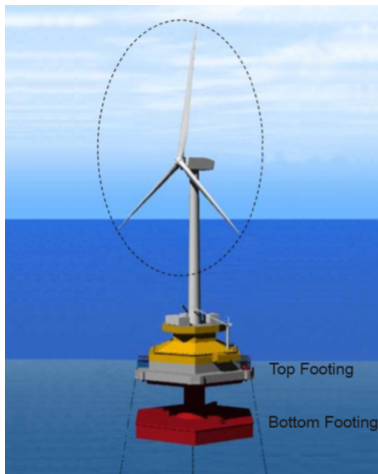
Figure 1. The conceptual idea of the Advanced Spar FOWT.
