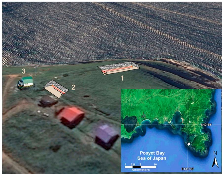
**Figure 3.** Number 1 is the 52.5-meter laser strainmeter, 2—17.5-meter laser strainmeter. 3—laboratory building.
