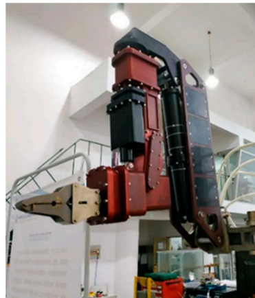
Figure 2. Deep-sea 6 d.o.f. electric manipulator.
