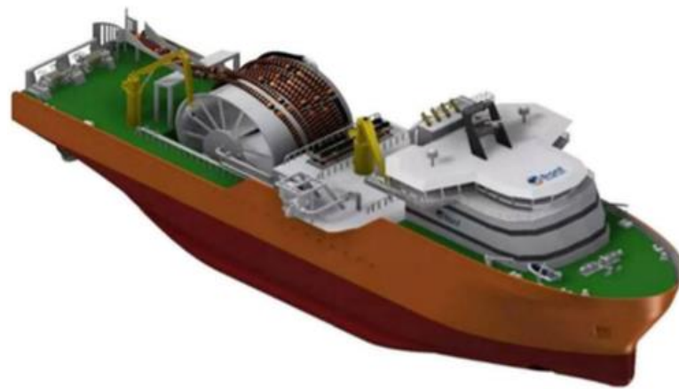
Figure 1. A cable laying vessel with DP system [3].
