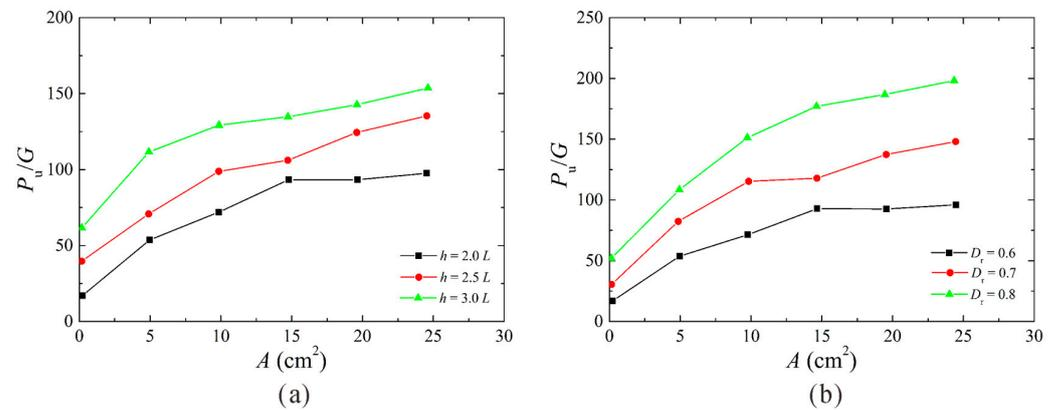
**Figure 10.**  $P$ – $A$  curves of the TAs under vertical pullout loading (a)  $D_r = 0.6$ ; (b)  $h = 2.0L$ .
