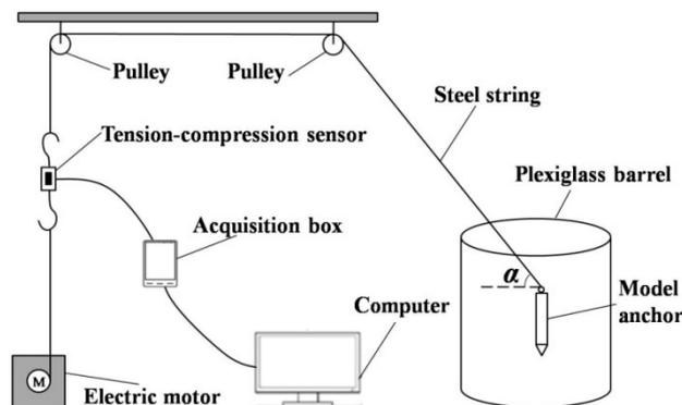
Figure 3. Schematic of the pullout test setup.
