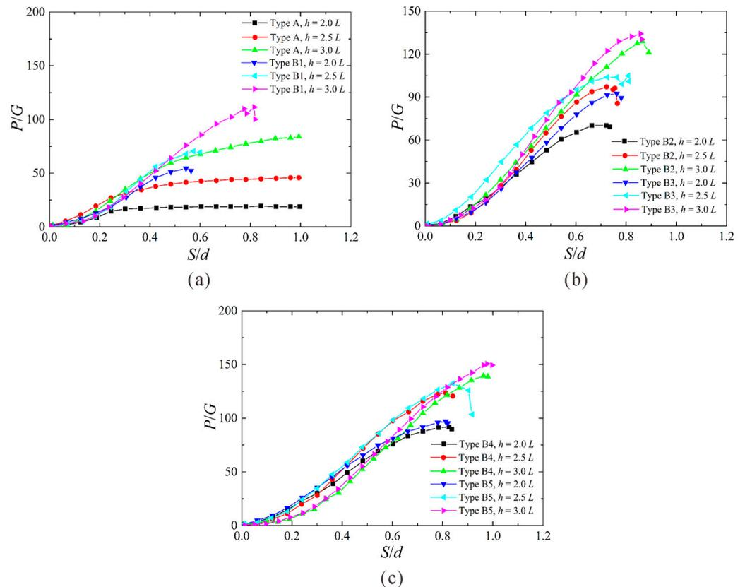
**Figure 6.** Effects of  $h$  on the load–displacement curves of the TAs under vertical pullout loading (a) Types A and B1; (b) Types B2 and B3; (c) Types B4 and B5.
