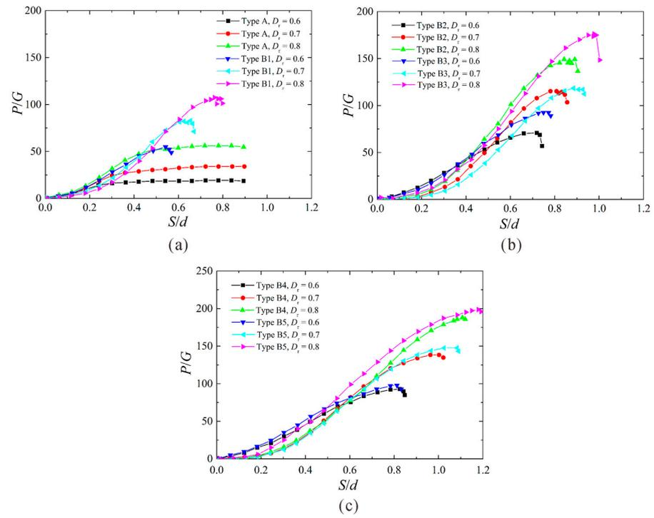
**Figure 8.** Effects of  $D_r$  on the load–displacement curves of the TAs under vertical pullout loading (a) Types A and B1; (b) Types B2 and B3; (c) Types B4 and B5.
