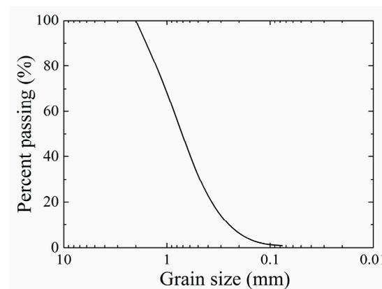
**Figure 1.** Particle-size distribution curve of the test sand.
