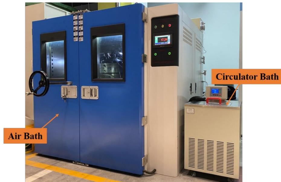
**Figure 6.** Air bath and water bath for DLCS temperature control.
