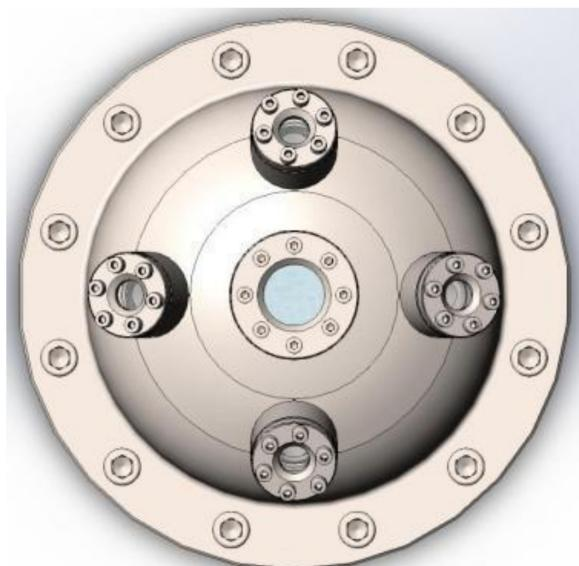
**Figure 5.** Schematic diagram of reactor cap.
