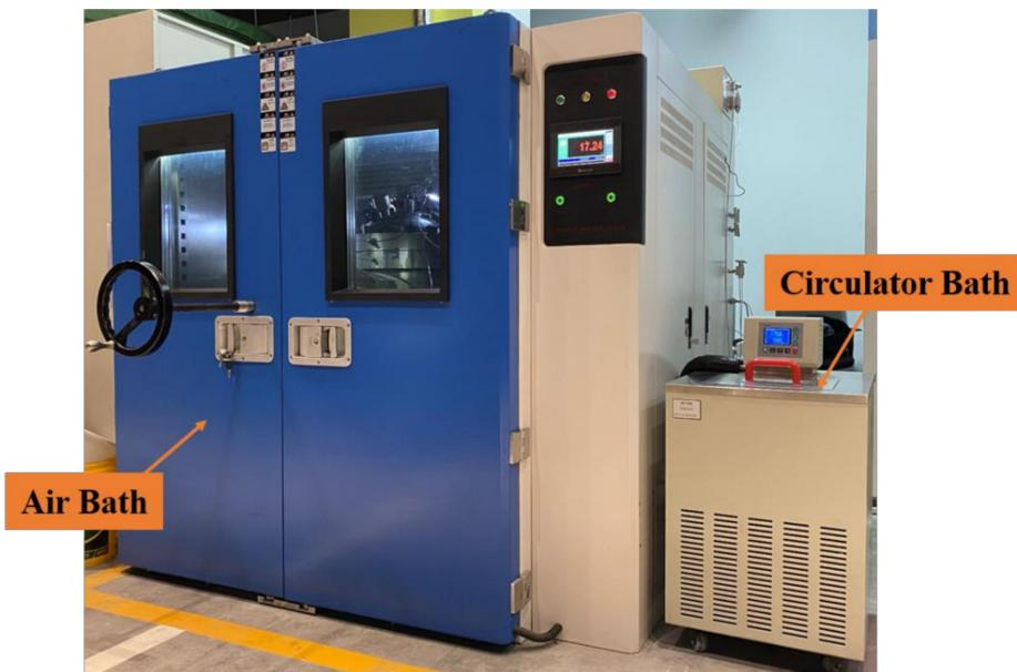
**Figure 6.** Air bath and water bath for DLCS temperature control.
