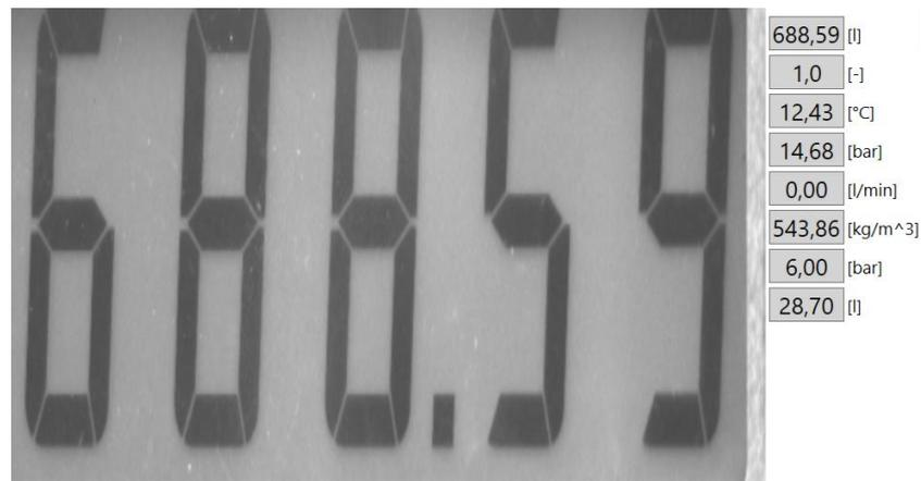
Figure 9. Software user interface when verifying the LPG dispenser.
