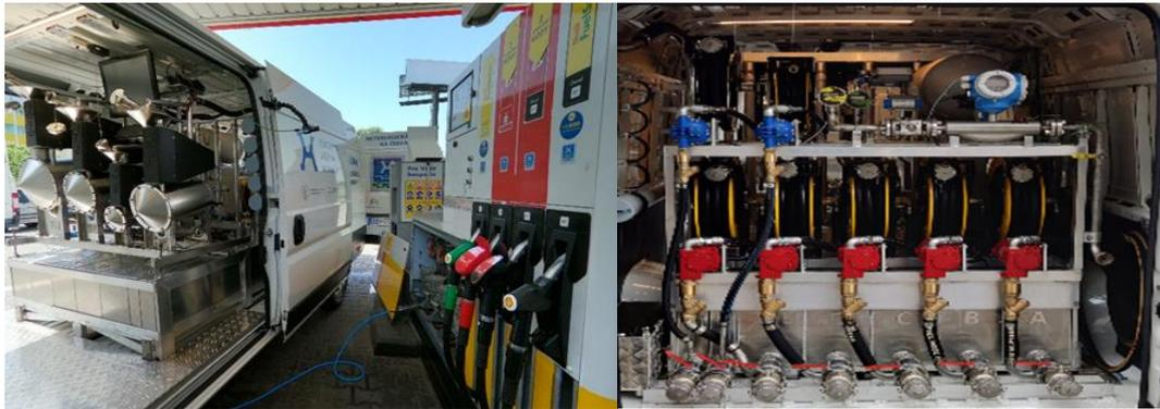
**Figure 1.** The AMSV system as a part of the conventional commercial vehicle up to 3.5 tones.
