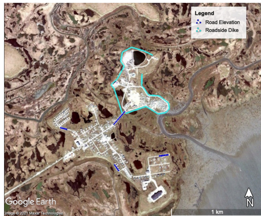
Figure 6. Planned roadside dike mitigation.
