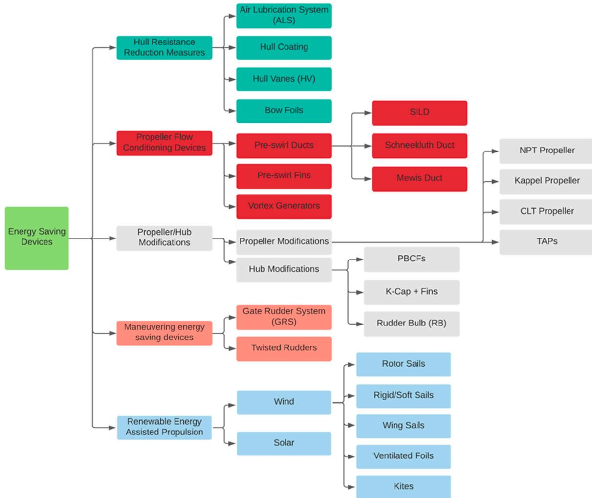
Figure 2. Categorisation of existing and emerging energy-saving devices (ESDs).
