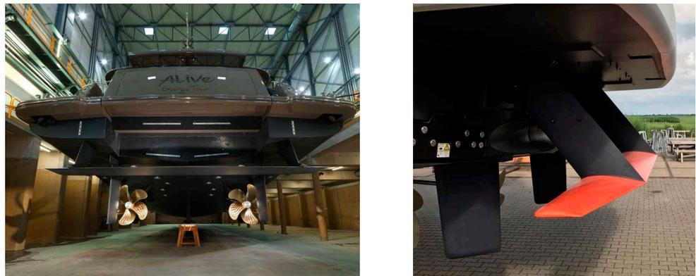
**Figure 6.** Hull Vane installation reproduced with permission; copyright Hull Vane.
