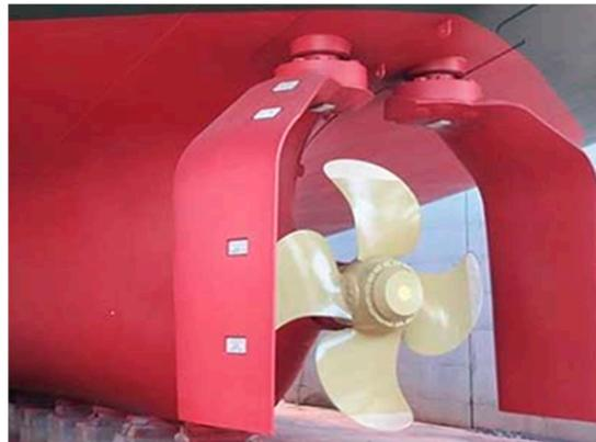
**Figure 11.** Gate rudder used in a sea trial, reproduced from [108] (CC BY).
