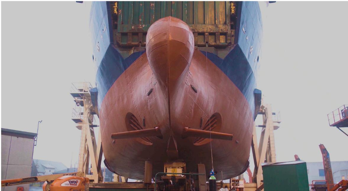
**Figure 7.** Wavefoil's retractable bow foil installed on ferry, M/F Teistin (Photo reproduced with permission; copyright Wavefoil).
