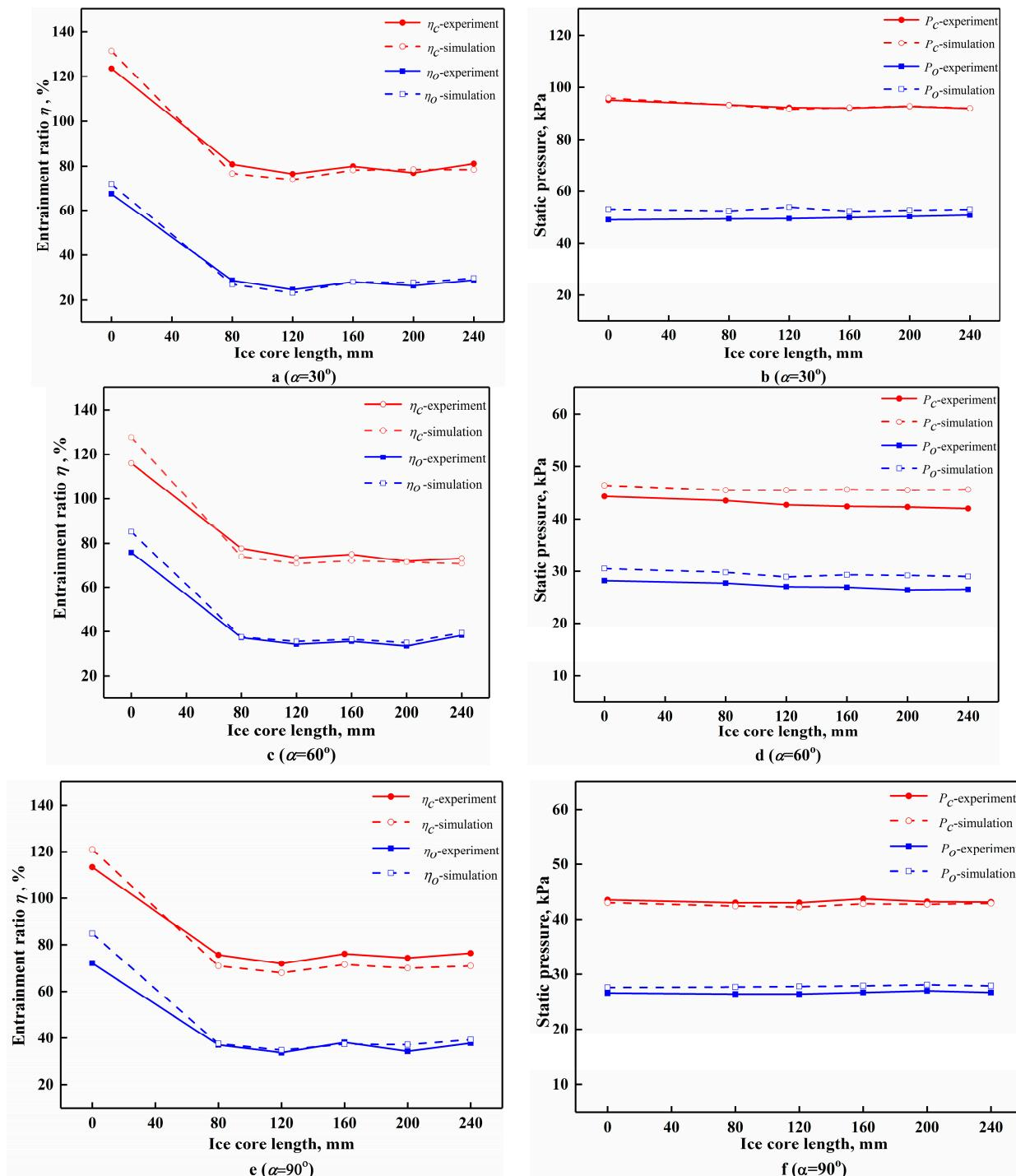
**Figure 5.** Comparison of simulation and experimental results. (a) entrainment ratio of  $30^\circ$ ; (b) static pressure of  $30^\circ$ ; (c) entrainment ratio of  $60^\circ$ ; (d) static pressure of  $60^\circ$ ; (e) entrainment ratio of  $90^\circ$ ; (f) static pressure of  $90^\circ$ .
