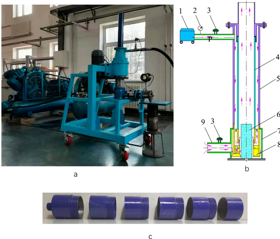
**Figure 4.** Equipment for testing ice drilling with air reverse circulation: (a) experiment table; (b) schematic; (c) ice cores; (1) air compressor; (2) pressure sensors; (3) vortex flow meter; (4) inner tube of drill bit; (5) outer tube of drill bit; (6) borehole wall; (7) ice core; (8) drill bit body; (9) suction tube.
