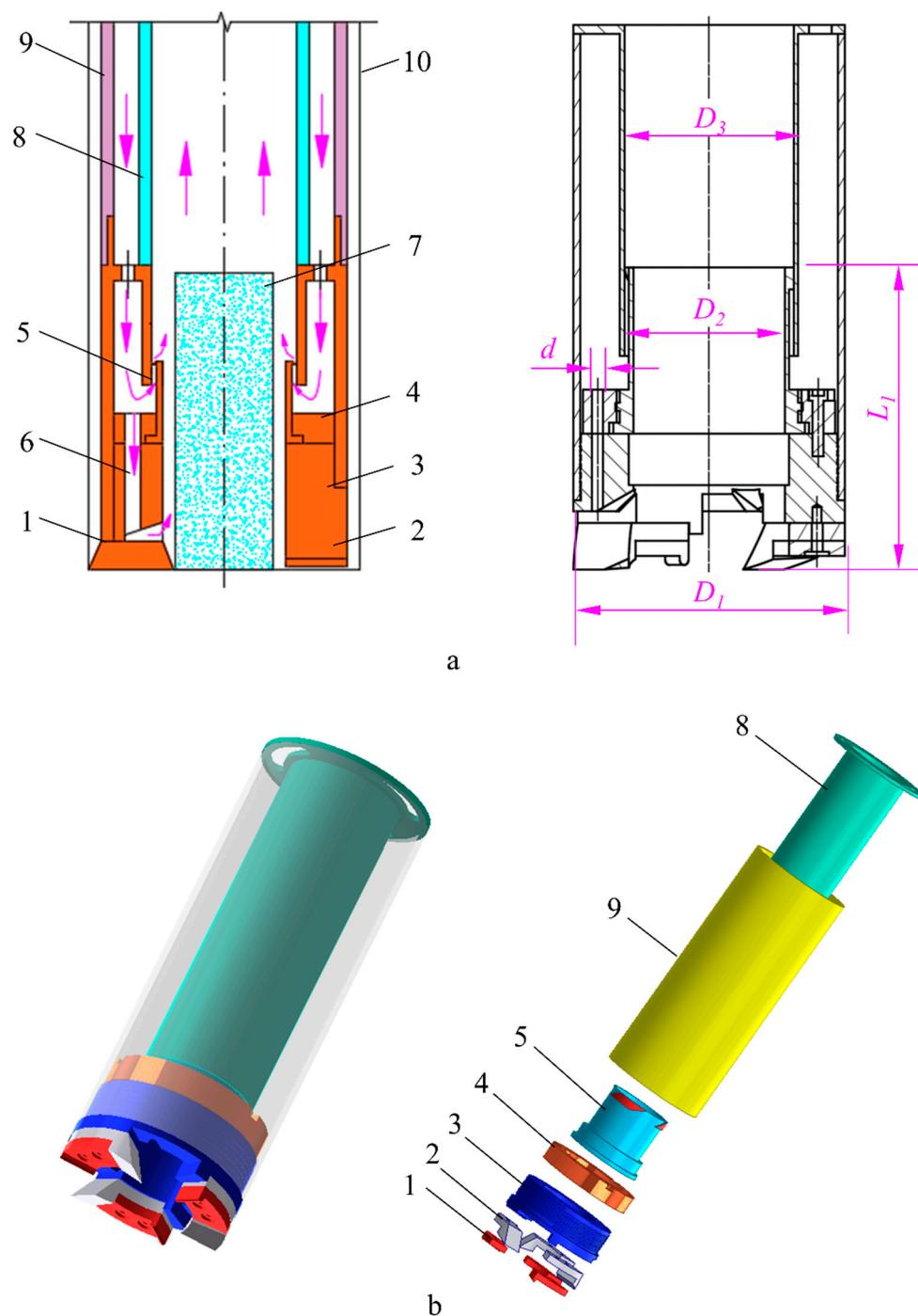
**Figure 1.** Swirling ice core drill bit: (a) working principle of the swirling drill bit; (b) 3D models: (1) cutters; (2) shoes; (3) lower drill bit body; (4) upper drill bit body; (5) swirler; (6) flushing nozzles; (7) ice core; (8) inner tube of drill bit; (9) outer tube of drill bit; (10) borehole wall.
