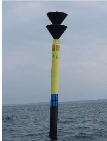
**Figure 11.** Spar buoy.
