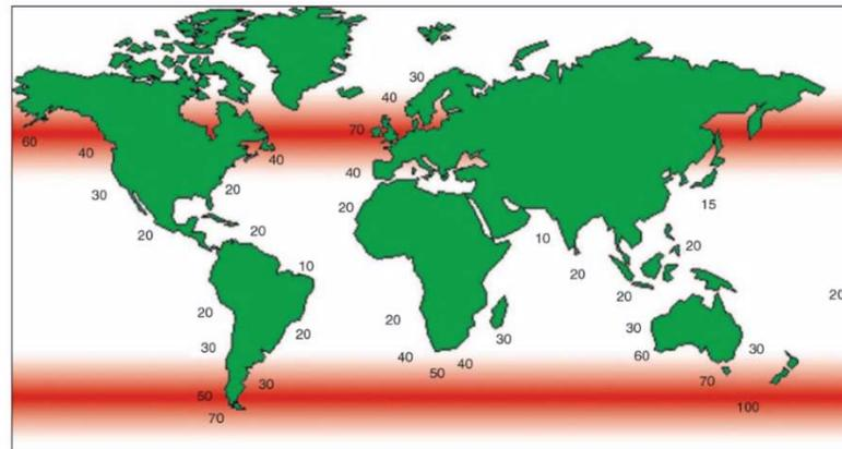
**Figure 1.** Global wave power distribution by kW/m of crest length (Centre for Renewable Energy Sources (CRES) [4]).
