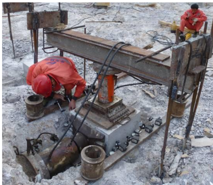
Figure 2. The in-situ direct shear test of the rock-concrete interface.
