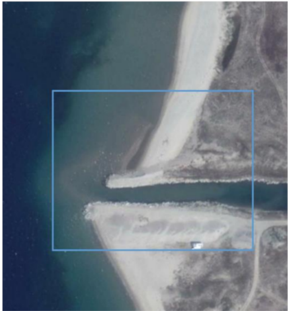
Figure 6. Ebb shoal developed by the sediment transport at the shelf side of the inlet induced by the ebb-dominated currents (Agiasma lagoon).
