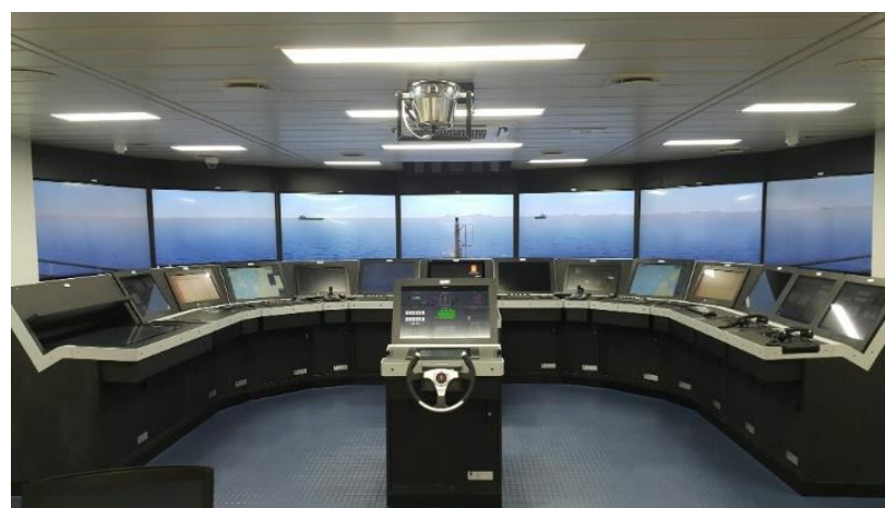
Figure 2. Full-mission-ship-handling simulator for the simulation experiment.
