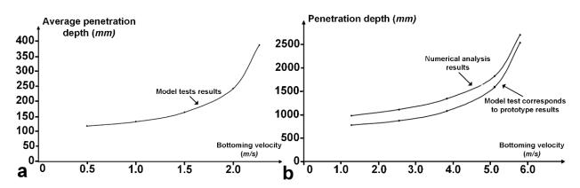
**Figure 13.** The penetration depth versus bottoming velocity of the anchor. (**a**) The results in the model test (**b**) The simulation results and the prototype results.
