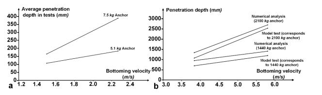
**Figure 14.** The penetration depth versus bottoming velocity and anchor weight. (**a**) The results in the model test (**b**) The numerical simulation results and the prototype results.
