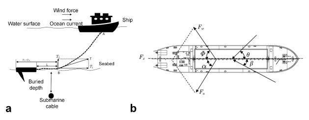
**Figure 3.** (**a**) The force acting on the ship and anchor when anchored. (**b**) The wind and hydrodynamic forces on the ship.
