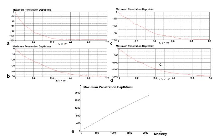
**Figure 7.** The maximum penetration depths of different anchor weights. (a) Case F1-1; (b) Case F1-2; (c) Case F1-3; (d) Case F1-4. (e) The relationship between the maximum penetration depth and the anchor weight.
