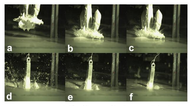
**Figure 11.** The different falling positions of the anchor in case F1-4. (**a**) The anchor is not touch the soil; (**b**–**e**) The anchor is penetrating the soil; (**f**) The anchor is in the maximum penetration depth.
