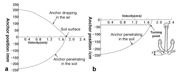
**Figure 12.** Dropping velocity versus dropping height and penetration depth. (**a**) The anchor dropping in the air and the soil. (**b**) The anchor penetrating in the soil and the turning point.
