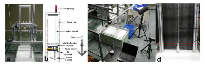
**Figure 10.** (a) The experiment platform, (b) height-adjustable anchoring platform, (c) high-speed image acquisition system, and (d) depth measurement module.
