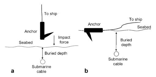
**Figure 1.** The impact and drag damage on submarine cables. (**a**) Impact damage on submarine cable; (**b**) Drag damage on submarine cable.
