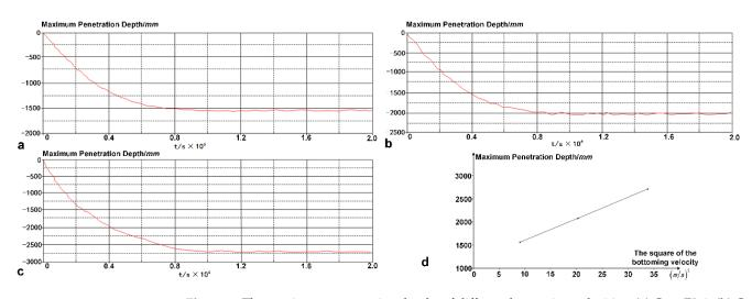
**Figure 8.** The maximum penetration depths of different bottoming velocities. (**a**) Case F2-1; (**b**) Case F2-2; (**c**) Case F2-3; (**d**) The relationship between the maximum penetration depth and the bottoming velocity.
