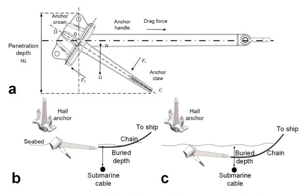
**Figure 4.** The drag force of the anchor in different states. (**a**) Force analysis of anchor dragging, (**b**) the anchor claw is submerged in the soil, and (**c**) the anchor crown is submerged in the soil.
