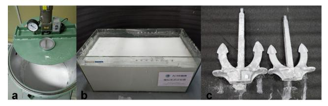
Figure 9. (a) The soil in vacuum stirring blender, (b) prepared soil in tank, and (c) model Hall anchor.
