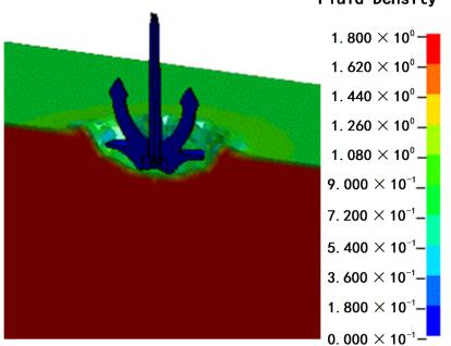
**Figure 6.** Numerical analysis of the penetrating process of the anchor in the soil.
