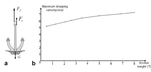
**Figure 2.** (a) The forces acting on the anchor when dropping in the water, and (b) the maximum dropping velocity of the anchor.
